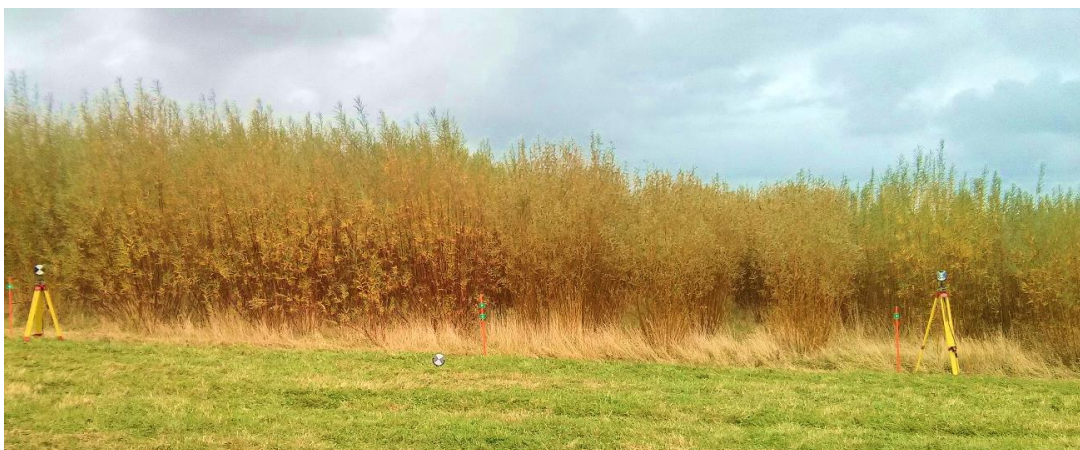
Figure 6-4. A view of the three plots covered from scanning position one, left is plot ‘E’, middle is plot ‘TE’, and right is part of plot ‘B’. Three out of four Leica black and white registration targets can be seen, in addition to the reflectors used to mark the approximate boundaries of each plot.
