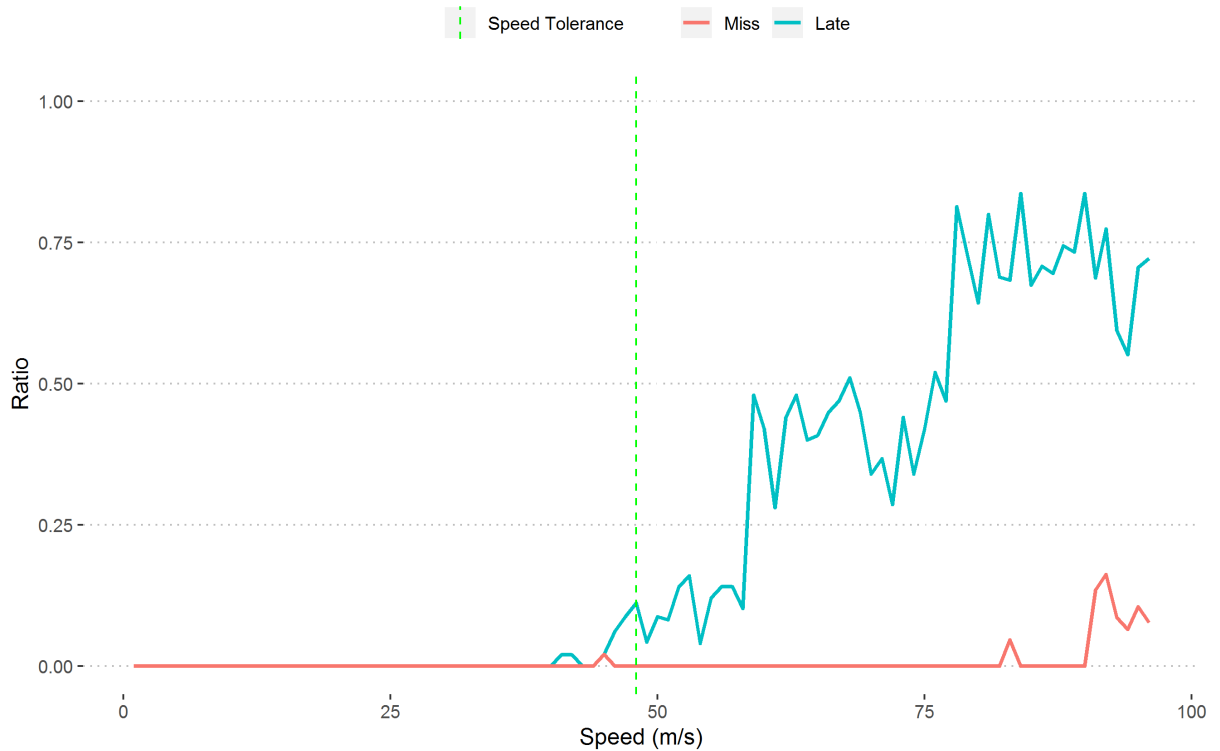
Fig. 5.24 Ratio of Late to Correct Collisions and Misses to Total Collision vs. Speed using a speed tolerance of 48\text{m}\cdot\text{s}^{-1} . The speed tolerance is marked in a dashed green line.
