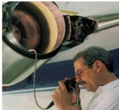
Figure 2.4 Illustration of visual testing of aircraft components using an endoscope by an operator [51].
