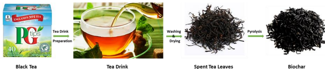
Figure 3.2. Schematic illustration of the biochar preparation from spent tea.
