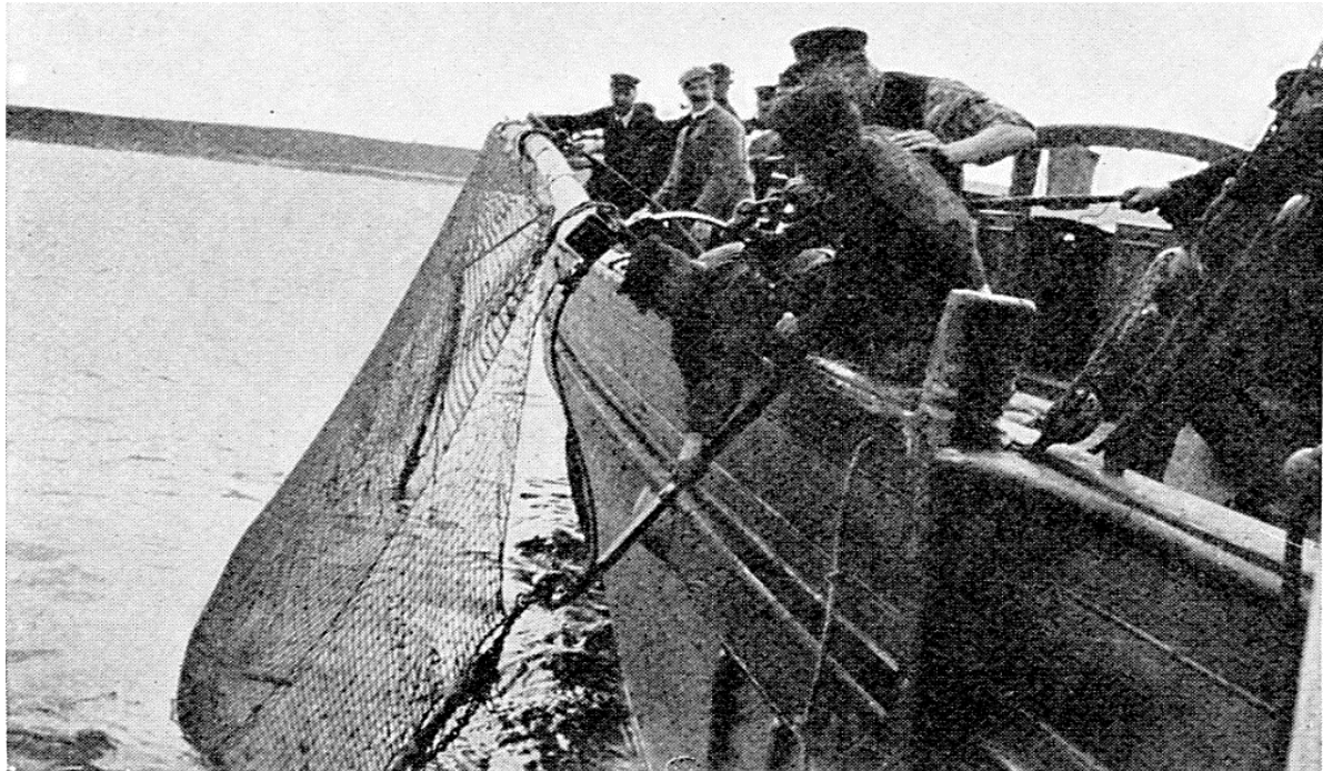
Figure 2.4. Photograph of the original 6.7 m beam trawl being hauled by members of the NSFC on the starboard side of the paddle tug Livingstone (Meek, 1899).
