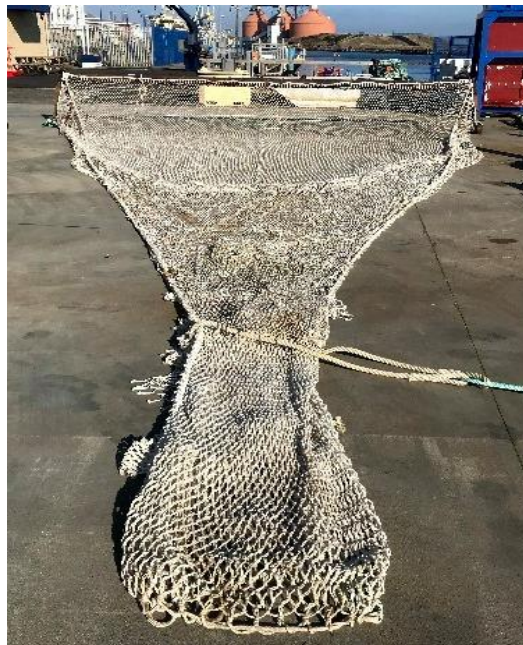
Figure 2.2. Detailed plan and photograph of the replica trawl net used to simulate the original net employed by the NSFC in the late 19 th century. Mesh numbers of individual panels are listed as 'front-width to back-width by depth'. Stretched inside meshes are given in mm. The codend was comprised of 3 mm double twine and remaining net panels of 4 mm single twine ( a = flapper; b = pockets).
