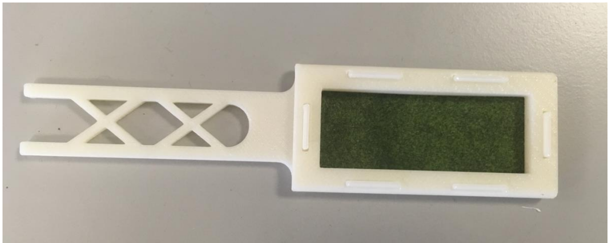
Figure 12: 3D printed scaffold used to secure the algae biocomposite paper for batch solutions.
