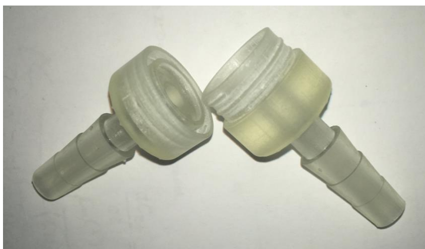
Figure 69: 3D printed connector that can be disassembled to house the algae biocomposite paper, for continuous flow adsorption/desorption metal experiments.
