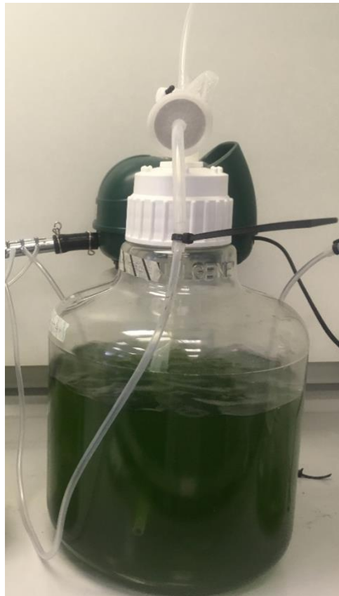
Figure 6: 10L Nalgene® carboy containing Synechococcus elongatus . The vented closure allows for air to be passed through the HEPA-VENT filter, and escape via a three-way stopcock. The Blagdon® KOY pond pump is shown in the background.
