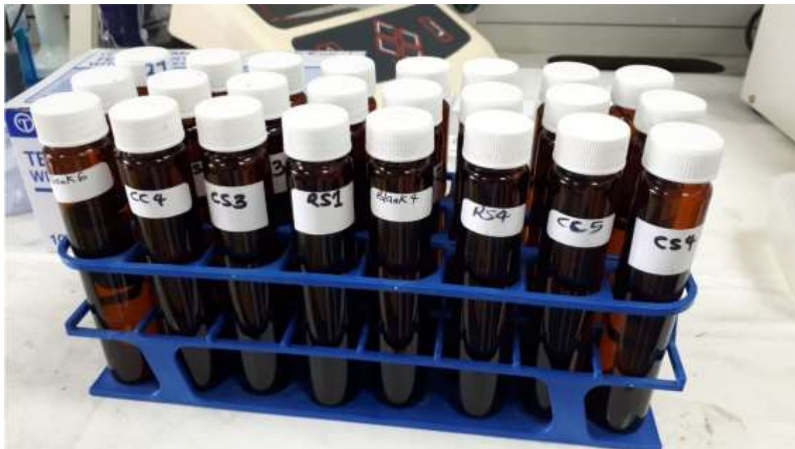
Figure 4-1. Batch experiments showing 60 mL amber vials with screw-top caps with PTFE liner.
