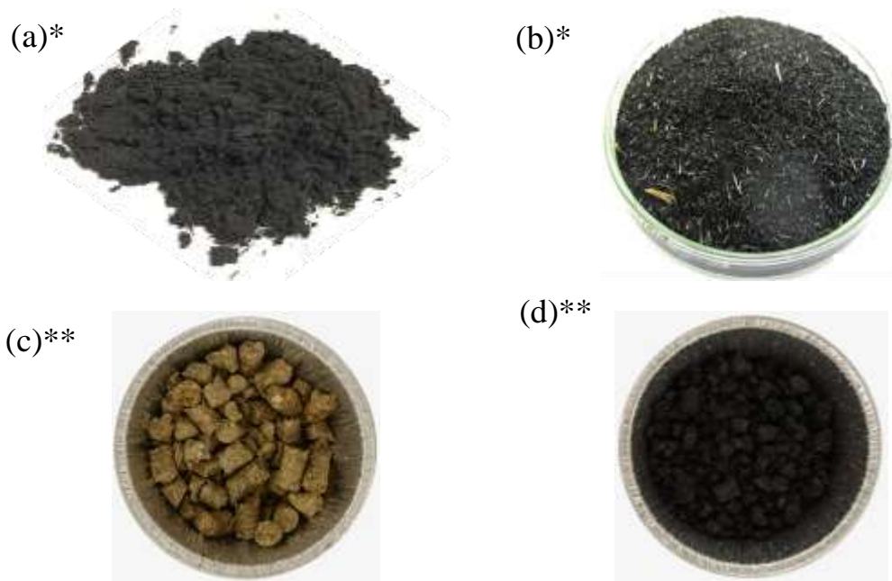
Figure 3-3. Soil amendment materials used in the study: (a) coconut shell biochar; (b) rice straw biochar; (c) wheat straw pellets; (d) wheat straw biochar. Sources: *images obtained from KMUTT **images are assessed from https://www.biochar.ac.uk/standard_materials.php
