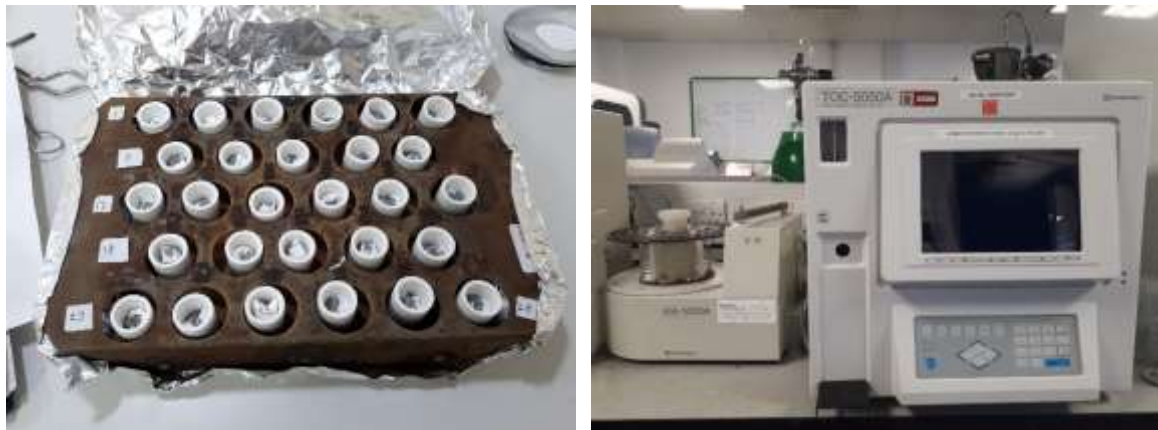
Figure 3-7 (a) Preparing samples for quantifying the particulate carbon (b) dissolved carbon analyser
