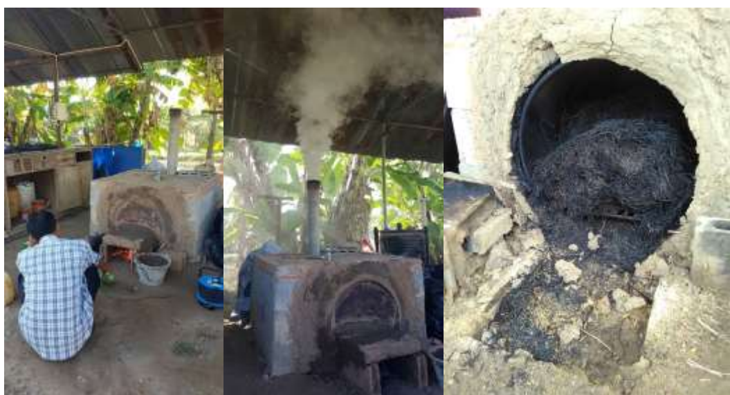
Figure 3-1. Biochars production using oil drum kiln and pyrolysis reactor (source: Energy and Environmental Engineering Center (EEEC), Kasetsart University Kamphaeng, Thailand).
