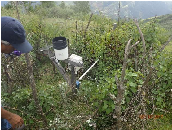
Figure 4-14 - Visiting a monitoring station in rural Sindhupalchowk, set up by Durham University. This records ground movement, in order to identify landslide hazards.
