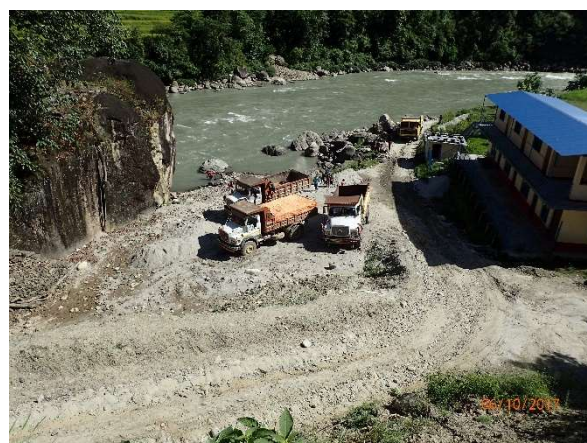
Figure 5-6 - Sand and gravel being collected from a river, next to an existing school, for use in local construction.
