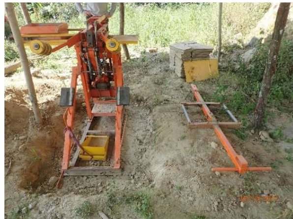
Figure 4-30 - A local brick-making factory in rural Sindhupalchowk. Entrepreneurs receive training in producing CSEB bricks, to be used in construction.
