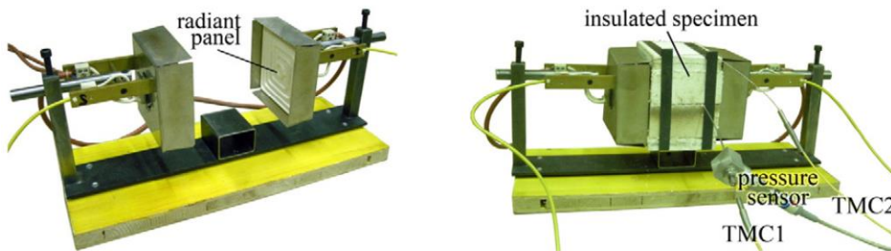
Figure 2.6 Schematic of the experimental set-up with the concrete slab (left); Schematic of the metal tube filled with a thermocouple and connected to a 'T-junction' (Right) (Kalifa et al. , 2000).
