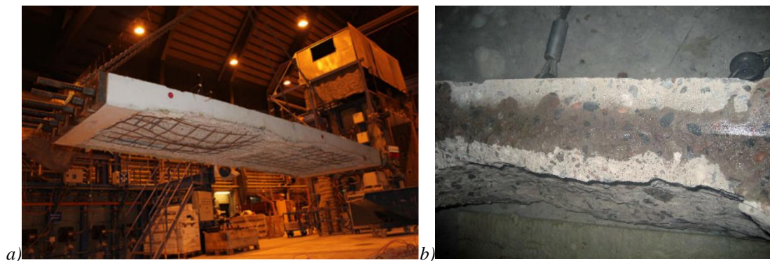
Figure 1.2 Concrete behaviours when exposed to high temperature: a) Concrete slab showed spalling and thermal expansion after the fire-spalling test ( www.tunneltalk.com ); b) Moisture content released from the concrete specimen when exposed to fire (McNamee, 2013).
