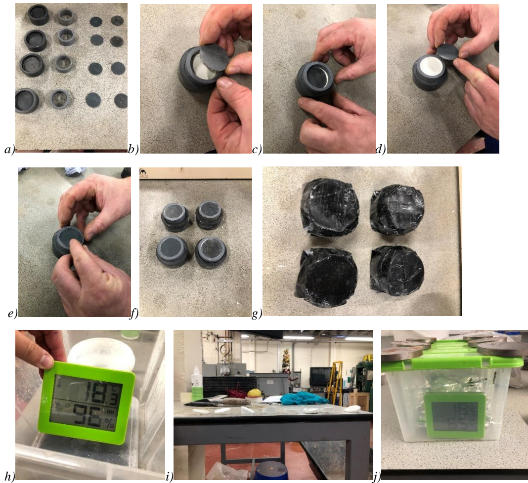
Figure 5.4 Schematic of casting specimens and storage condition: a) specimen mould, b) - f) casting specimens, g) sealed samples, h) the specimens curing condition (the white plastic jar filled with deionised water), i) all specimens after 28 days curing, j) pre-equilibrating all specimens at 60% by using saturated \text{NH}_4\text{NO}_3 salt solution.
