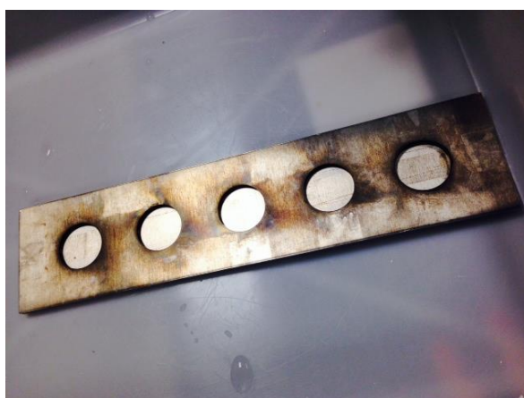
Figure 3-2. Steel mould for phase inversion membranes.
