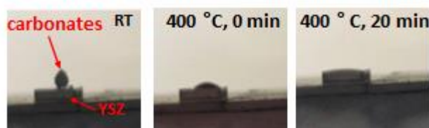
Figure 5-9. Wetting experiment with the YSZ single crystal/molten carbonate system. Heating was conducted under pure Ar in a controlled atmosphere furnace.
