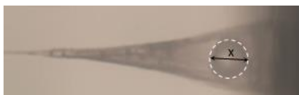
Figure 5-10. The determination of the size of the bubble formed inside the melt of the single pore in the \text{Al}_2\text{O}_3 single crystal using the two-dimensional image of the camera.
