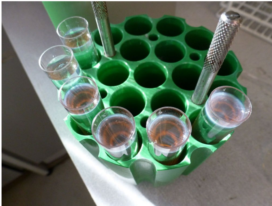
Figure 2.3 VLDL1 - TG appears as a milky colour ring top layer on the top of the test tube.
