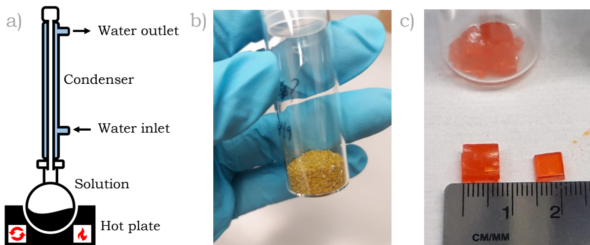
Figure 2.1: a) Reflux setup. b) \text{Cs}_3\text{Sb}_2\text{Br}_9 crystals. c) \text{MAPbBr}_3 single crystals.
