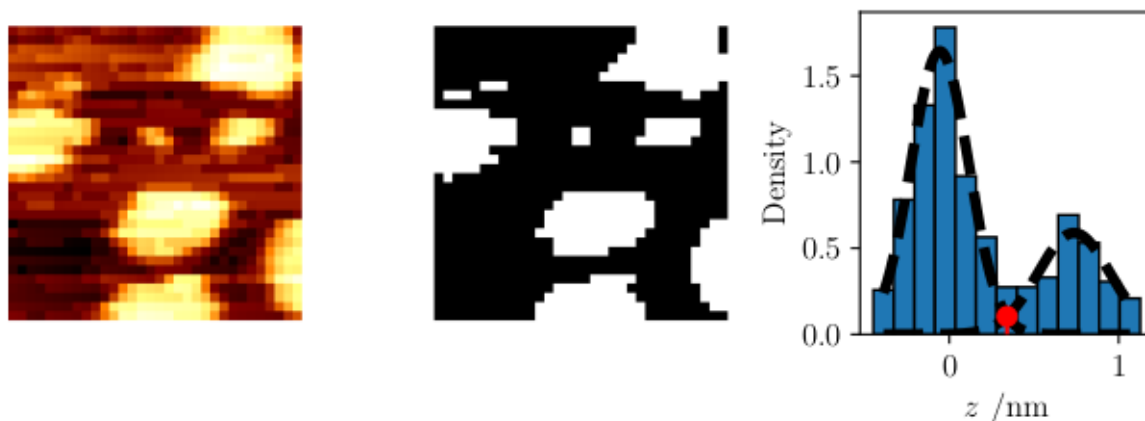
Figure 3.2: Contact mode image of a one of the segments analysed for determining raft height in the DOPC/DPPC SLB (A) with a binary mask applied (B) based on the z value indicated in the probability density of z values (C). The two Gaussian fits have been indicated with black dashed lines. The binary mask is shown for confirmations of raft identification only and not used in calculations further.
