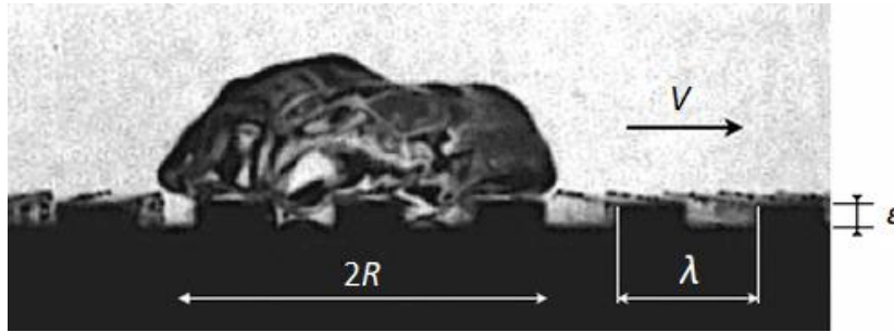
Figure 2.14 – Crenelated surface stops a moving droplet. Figure taken from Dupeux et al.
