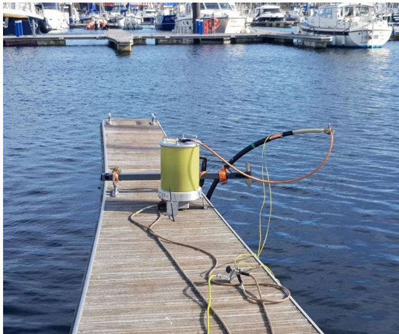
Figure 7- 18: Open Water Trial Test Setup – Live PD Occurrence through Cable Sample Testing
