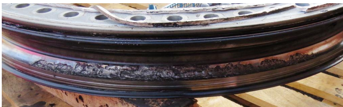
Figure 7.1 A fatigue fracture failure phenomenon of slewing bearing
