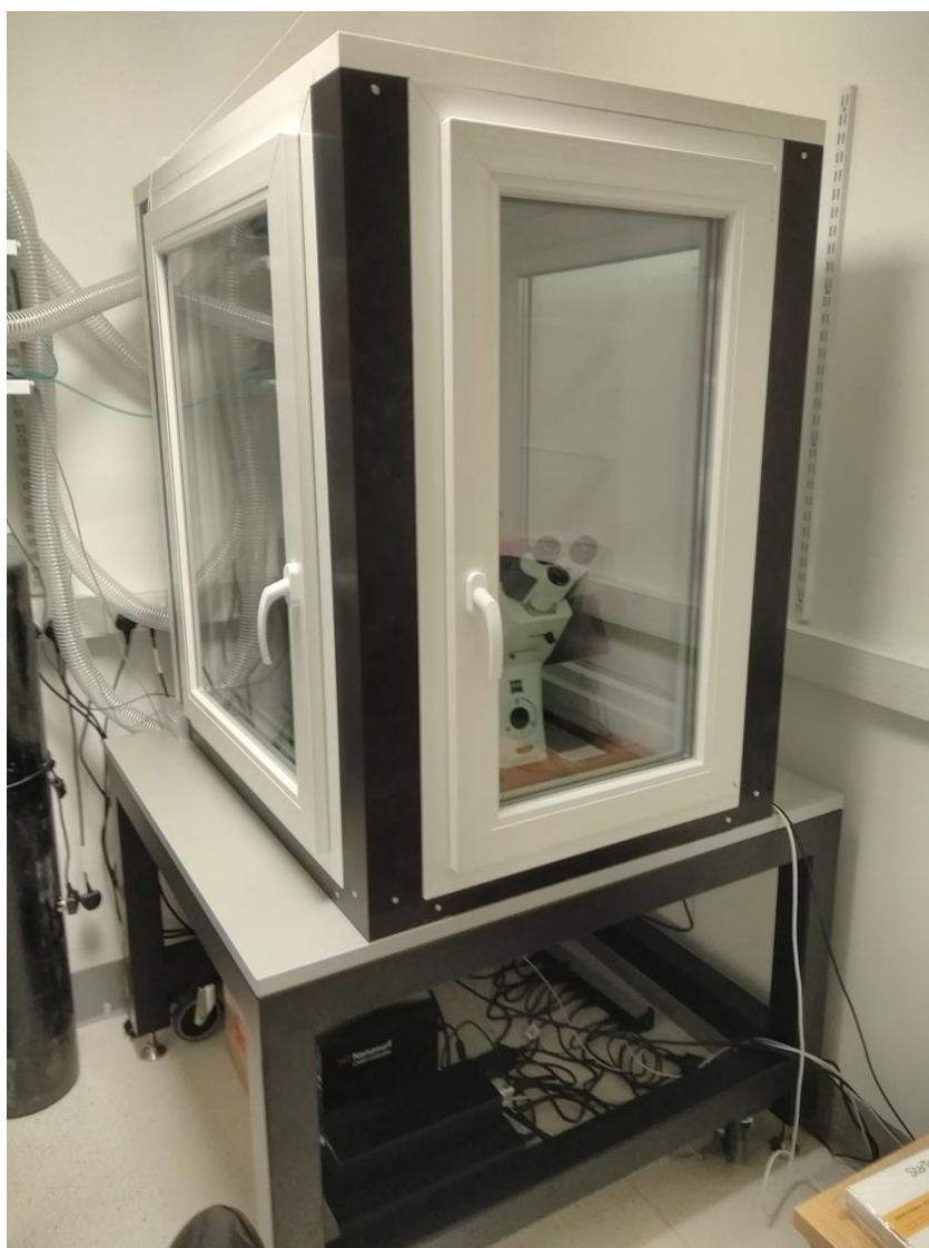
Figure 4-1. AFM-based FluidFM system consisting of an AFM, inverted microscope, pressure controller, vibration-resistant platform, and environmental isolation chamber.
