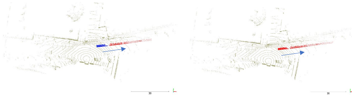
Figure 4.14. Vehicle example 10 from Study Site 2. Left: trajectories from the tracking-by-detection method; right: trajectory from the proposed method.
