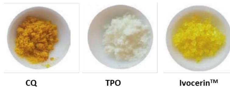
Figure 10: Initiators used for dental composite polymerization.
