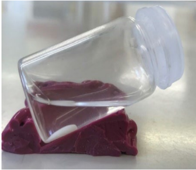
Figure 41: Specimens of dental composites stored in liquid at 37 °C. In this case, the specimen is stored in distilled water to detect fluoride release.
