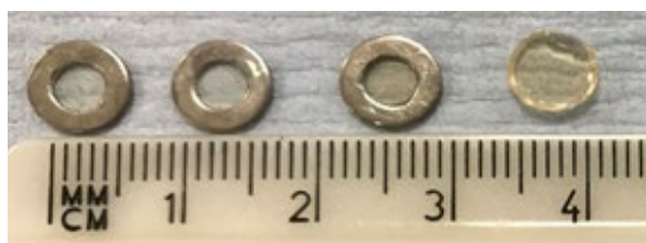
Figure 28: Metal molds used to prepare composite samples.
