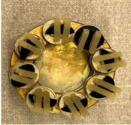
Figure 44: Composite specimens on SEM stubs applied with sticky carbon, ready to be gold coated for SEM images.
