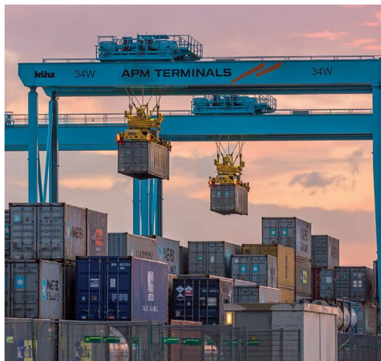
Figure 2.2: Automated Stacking Crane (ASC) at Port of Rotterdam Source: Kuenz cranes.
