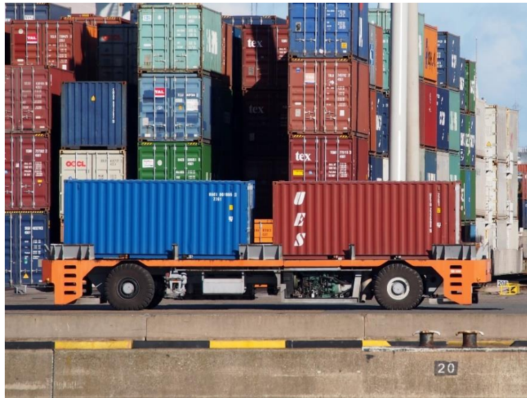
Figure 2.1: Automated Guided Vehicle (AGV) container mover at Port of Rotterdam Source: Wikipedia Commons.
