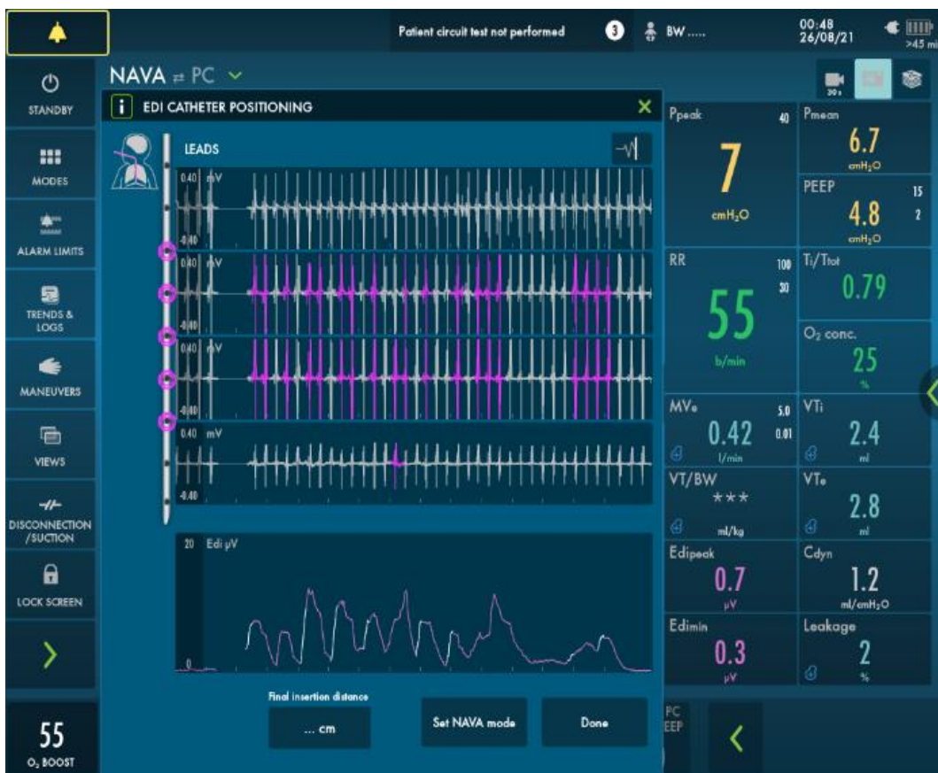
Figure 2.2 Edi catheter positioning screen showing optimal catheter position. The ECG signal decreases in amplitude from the upper to lower leads, and the pink EMG signal is highlighted in the central leads.
