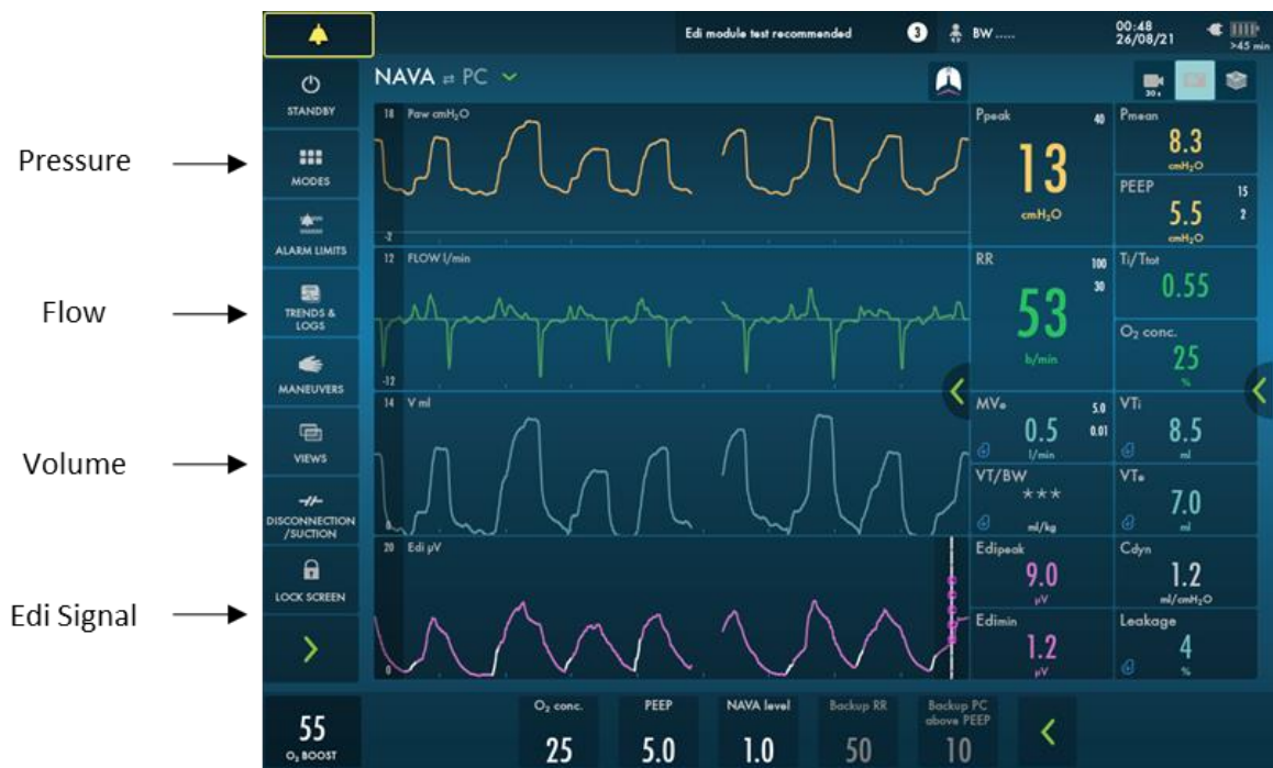
Figure 1.6 Neurally adjusted ventilatory assist (NAVA) screen showing diaphragm electrical activity (Edi) signal (lower pink trace) and delivery of positive pressure, flow, and volume in synchrony with and proportion to this.
