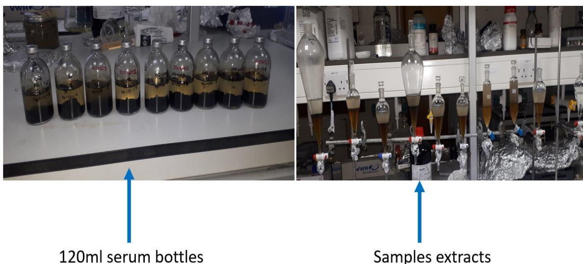
Figure 0.1: Anaerobic biodegradation experimental set up.
