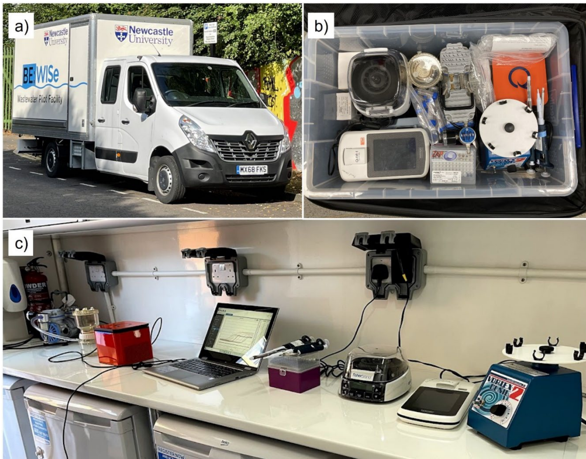
Figure 3.1. a) Mobile laboratory in the back of a van; b) the equipment items needed for onsite marker gene quantification inside a suitcase for transportation, and c) the equipment items set up on the bench of the mobile laboratory, from left to right: Vacuum pump, filtration unit, qPCR instrument, laptop computer, pipettes and tips, centrifuge, fluorometer and vortex with adapter.
