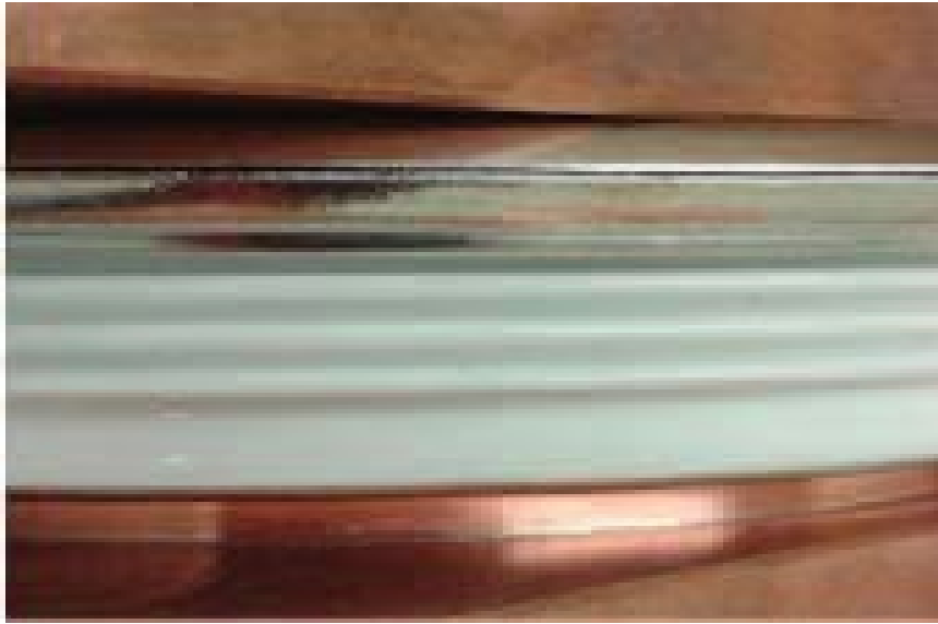
Figure 2.12 Collector electrode warpage [13]
