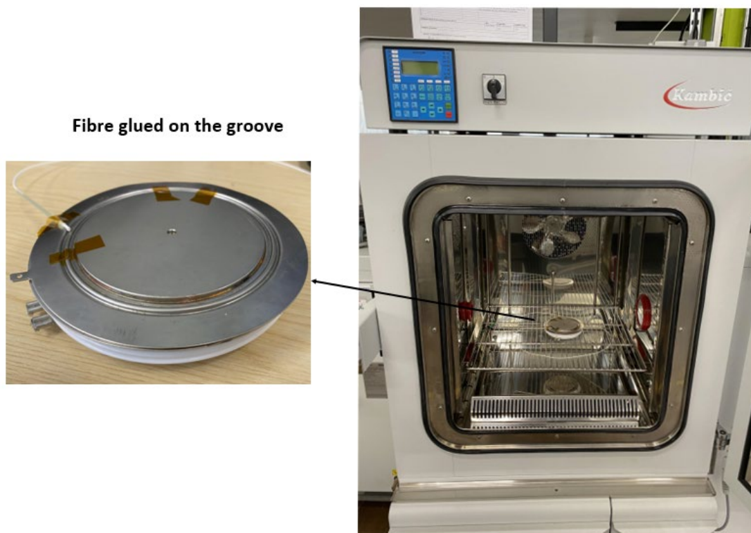
Figure 5.5 FBG fibre install on the lid groove with EP310 in the environmental chamber
