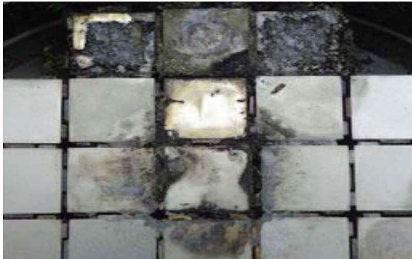
Figure 2.11 Failed Mo plate and IGBT chips [13]
