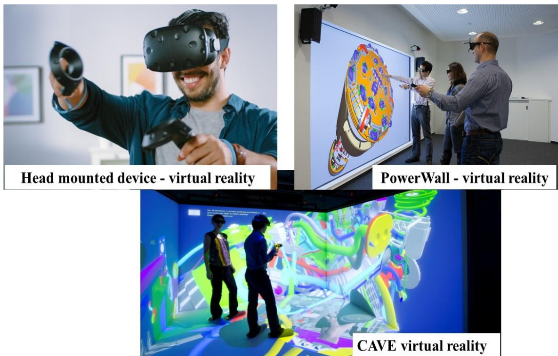
Figure 2.2: Pictures of a man wearing a VR head-mounted device with hand controllers, a group of people experiencing VR via a PowerWall projection, and two people in a CAVE environment.
