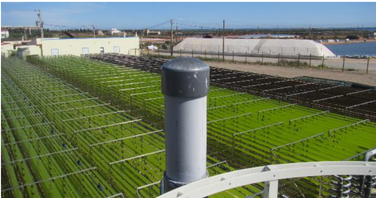
Figure 5-2: Photobioreactors at the Necton site in Olhão, photograph by author. The green photobioreactors (left) contain nannochloropsis salina , and the brown (right) contains phaeodactylum tricoratum .
