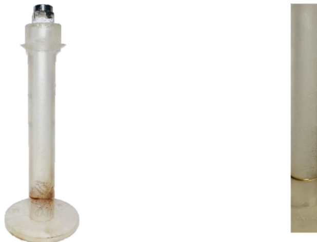
Figure 6.2. An example photo of a 3D-printed MFB that has deformed and cracked during packed-bed regime heating only due to possible localised high-temperature spots.
