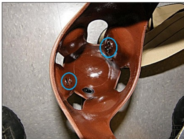
Figure 7.2: The inside of a compression-release socket featuring EMG sensors, highlighted in blue circles, mounted within the compression struts. Image from [25].
