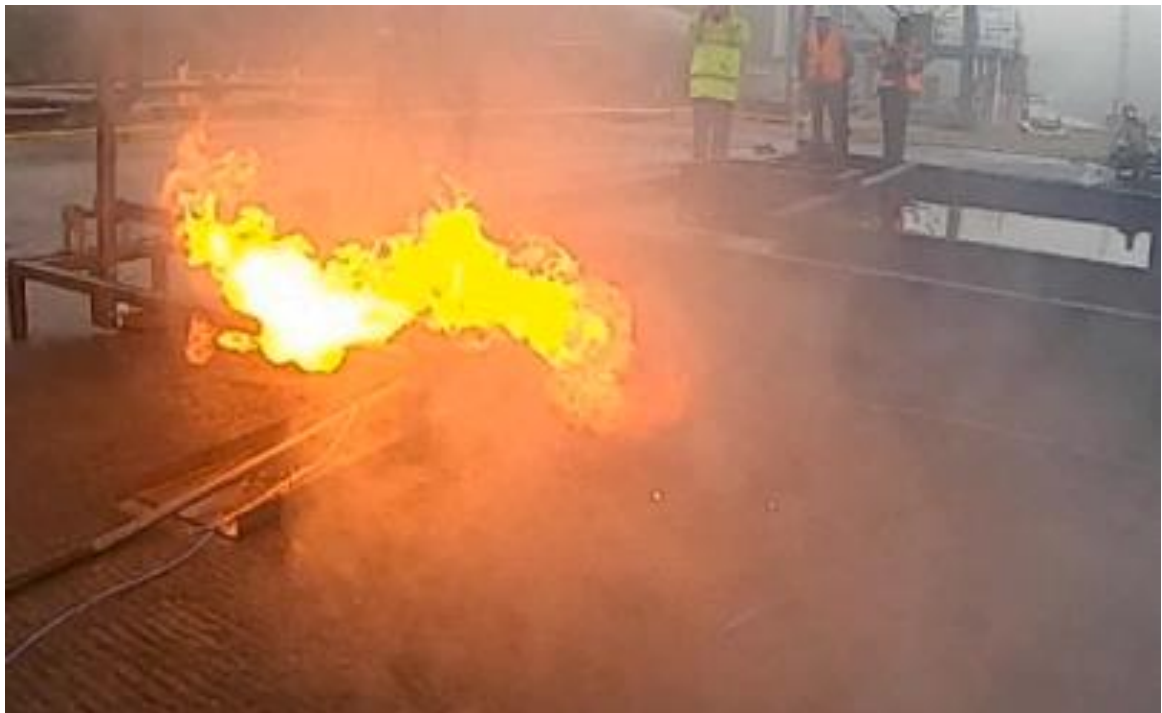
(h) The ignition of the white vapour spreads and a thinner fume from the module is observed (time = 13.4 s).
