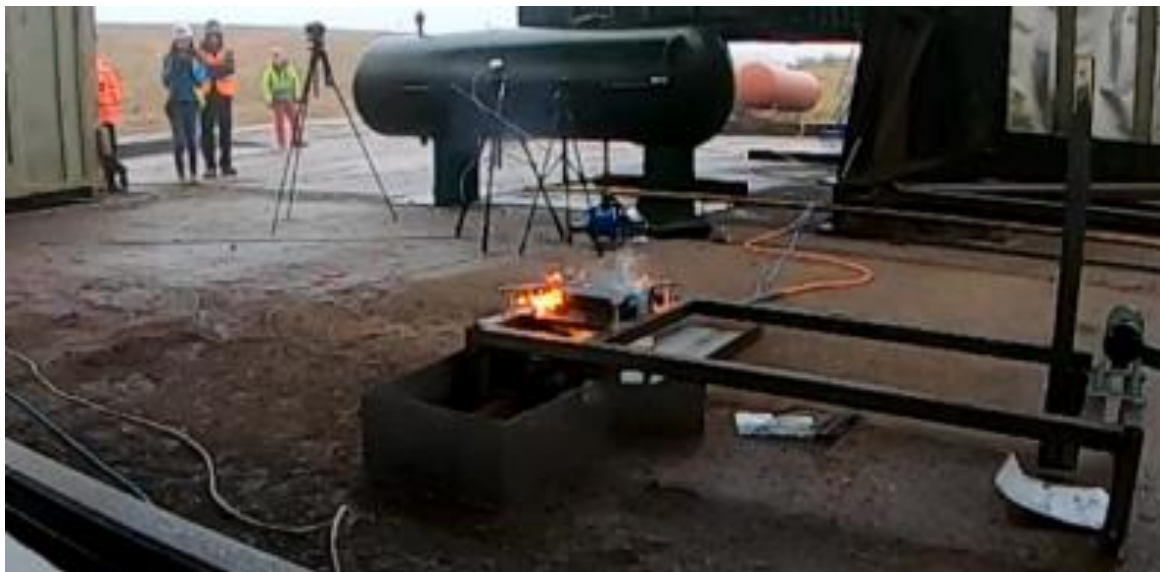
(a) Small flames are first observed 46 s after the introduction of the burner.
