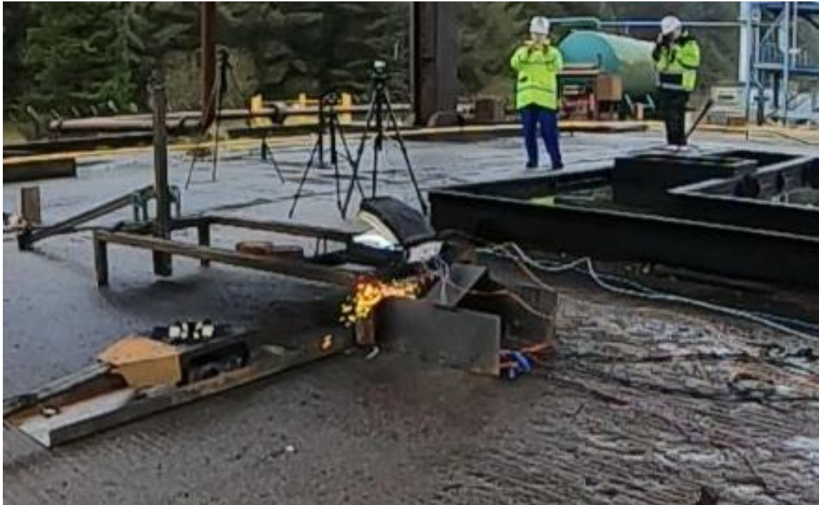
(e) A photograph of the front of the module when the flame front detaches (time = 57.5 ms).
