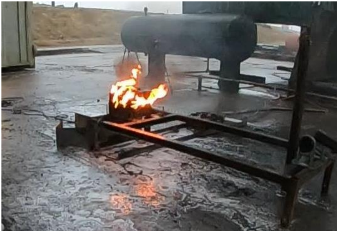
(n) A photograph of the rear of the modules as it re-ignited (time = 238 s).
