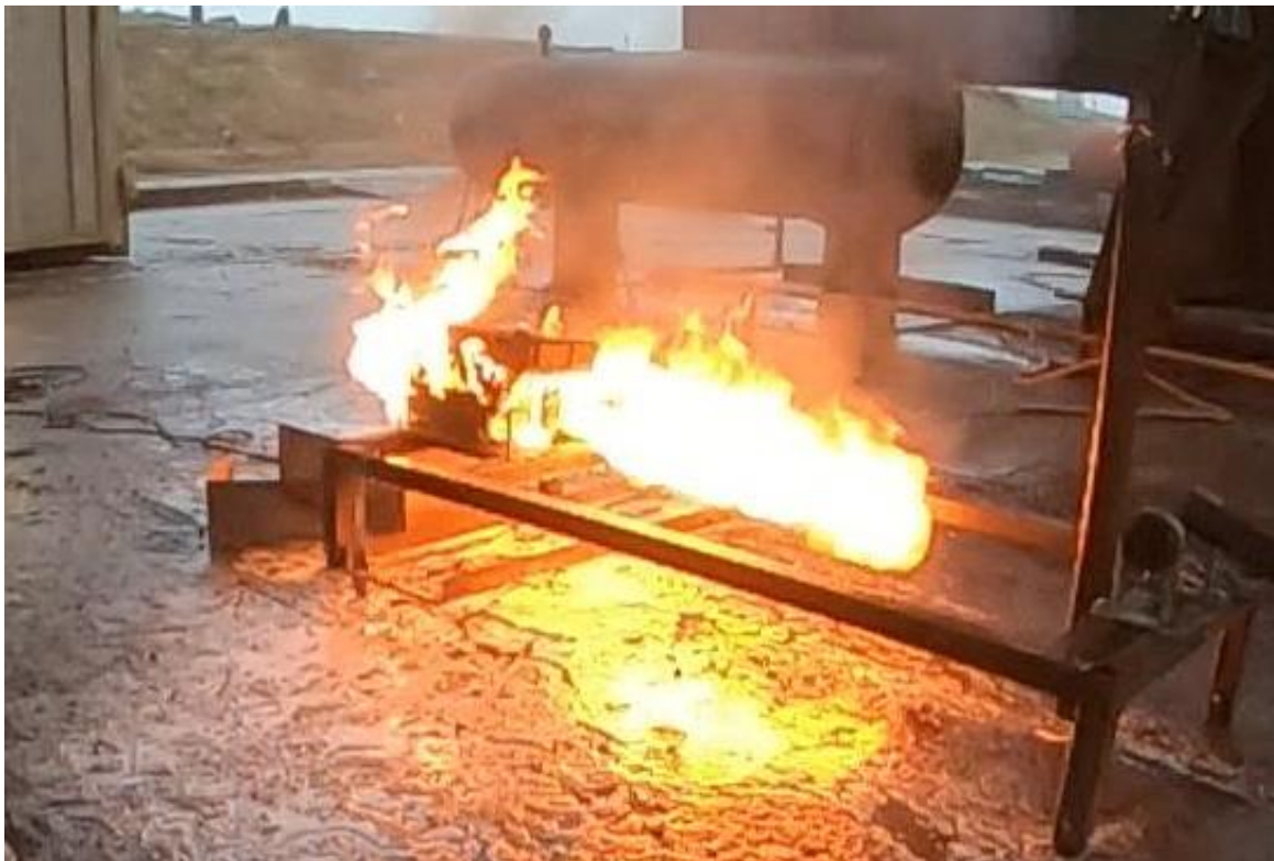
(p) A photograph of the rear of the modules as flare-like flames were re-produced after extinguishments (time = 257 s).
