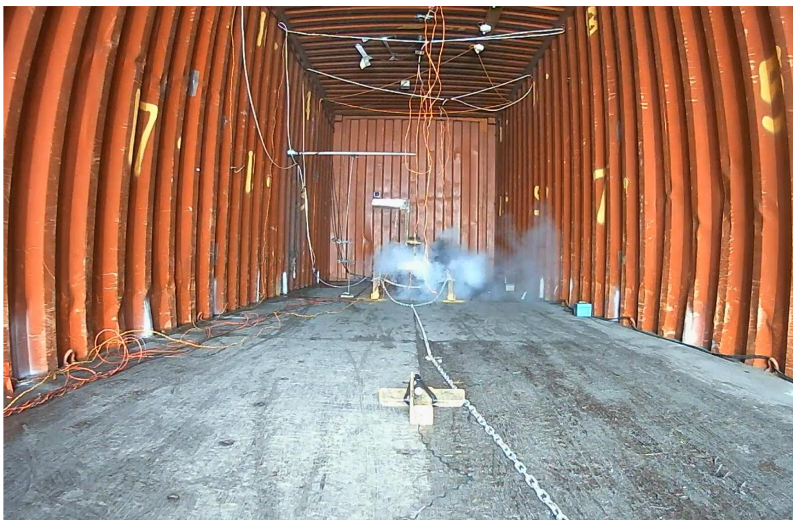
(c) A photograph taken during experiment C4 when the nail rose out of the module (time = 10.2 s).
