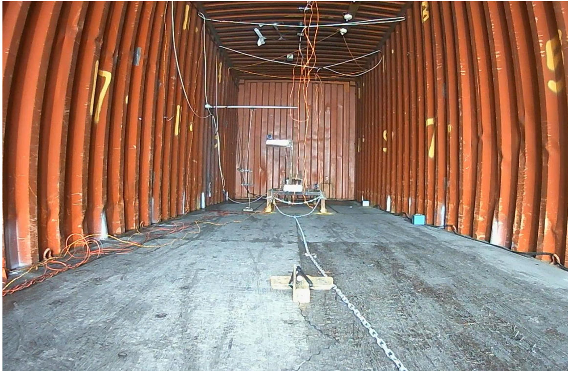
(a) A photograph taken during experiment C4 when the nail first penetrates the module (time = 0 s).
