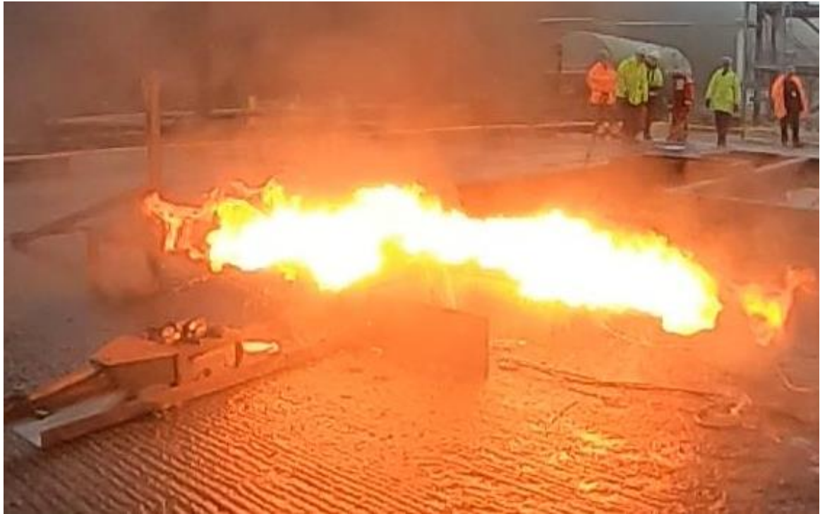
(i) A photograph of the front of the modules when flare-like flames were observed (time = 46.2 s).
