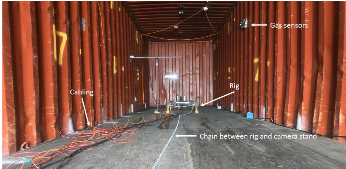
Figure 2.17. A photograph of the experimental setup at DNV 2.
