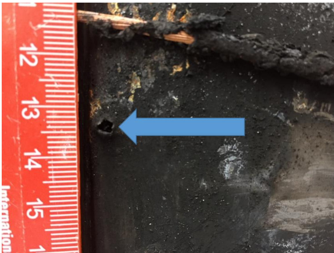
Figure 3.5. A photograph of the underside of the module employed in experiment A2, showing the exit hole (arrowed) of the nail.
