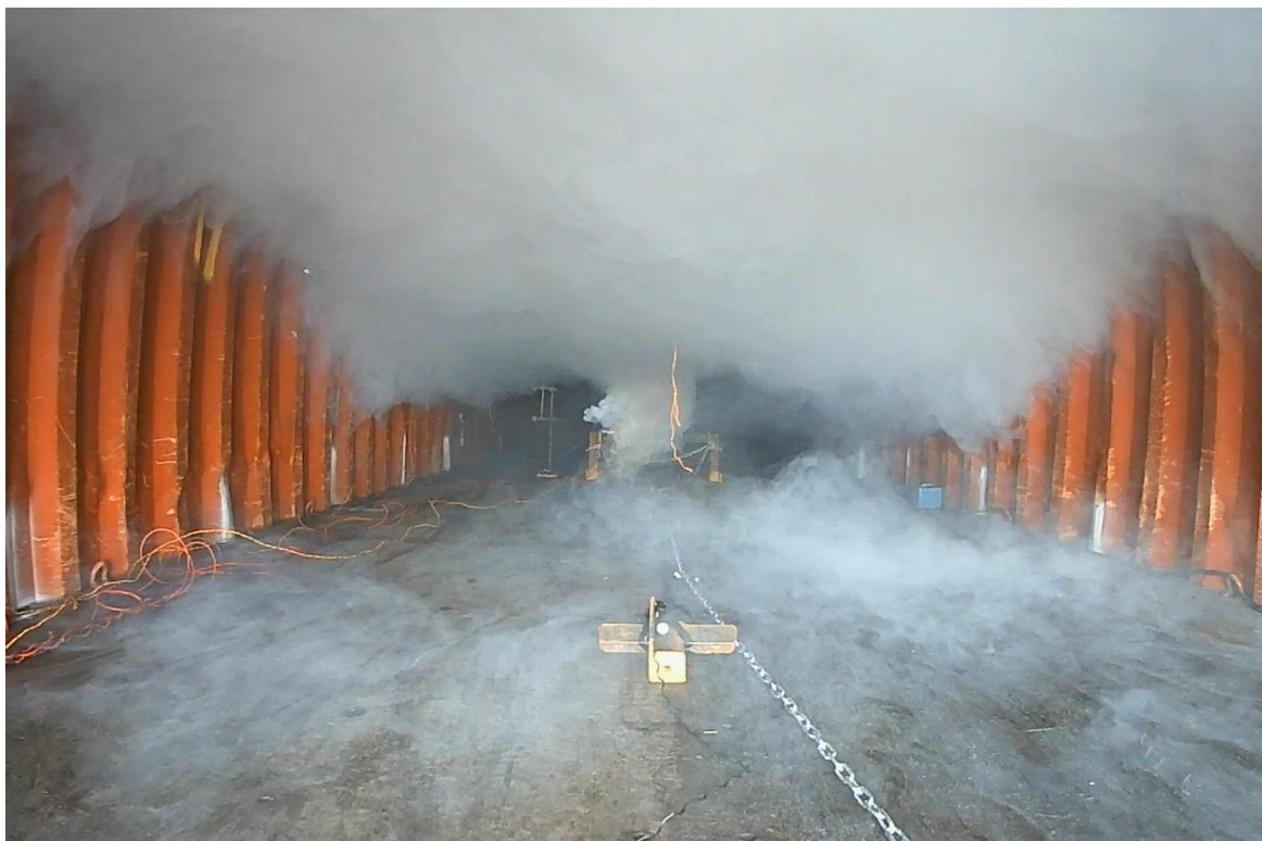
(f) A photograph taken during experiment C4 when the heavier than air type vapour cloud accumulates on the floor of the container (time = 85.4 s).
