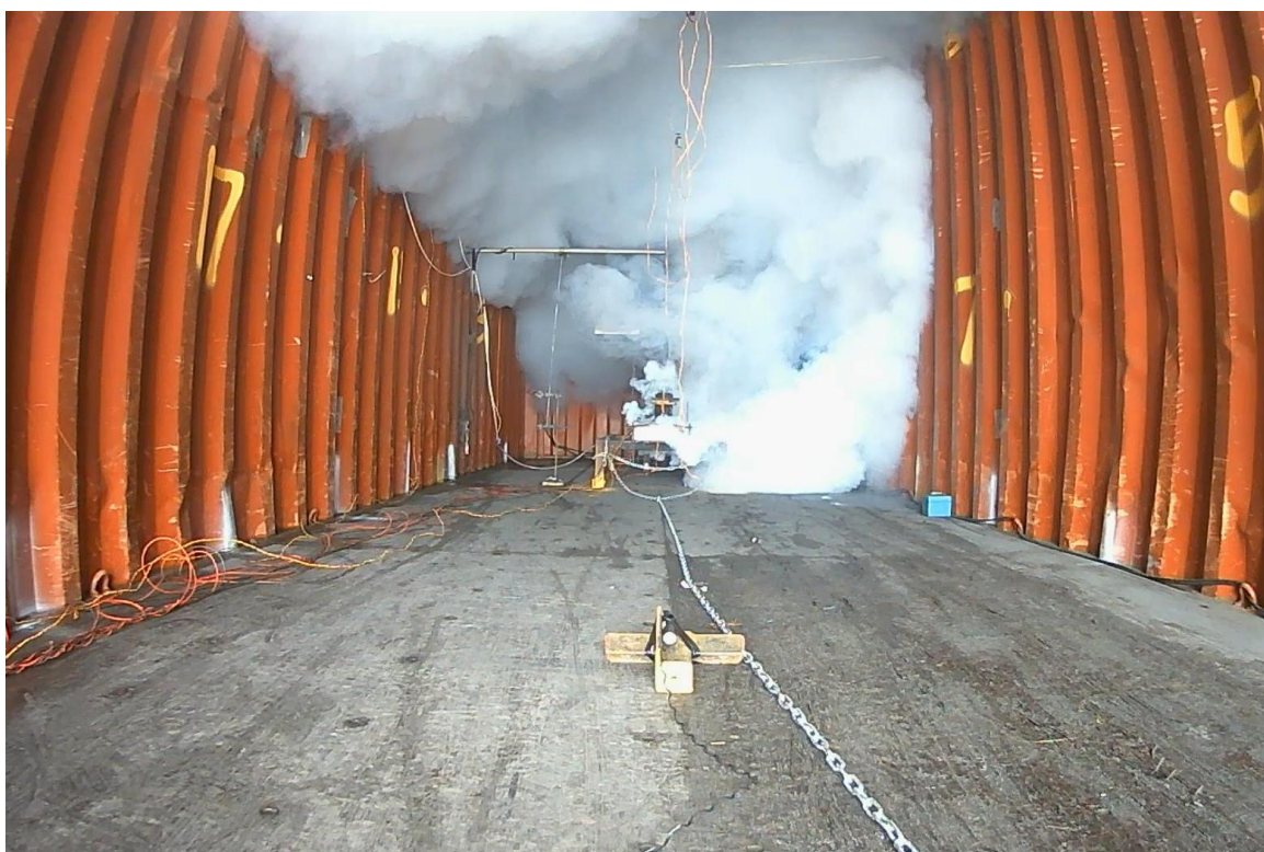
(d) A photograph taken during experiment C4 when there was an explosive release of black material, presumably nanoparticles from the cathode, and the white vapour accumulates on the ceiling of the container (time = 27.2 s).
