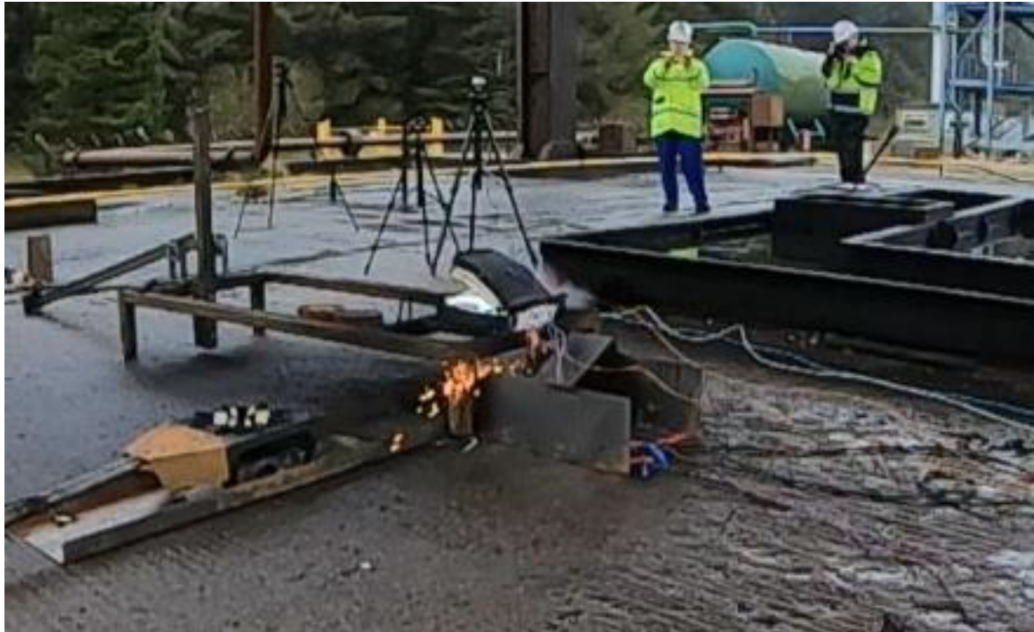
(g) A photograph of the front of the module when the first spark of the rear of the module can be seen (time = 95.8 ms).
