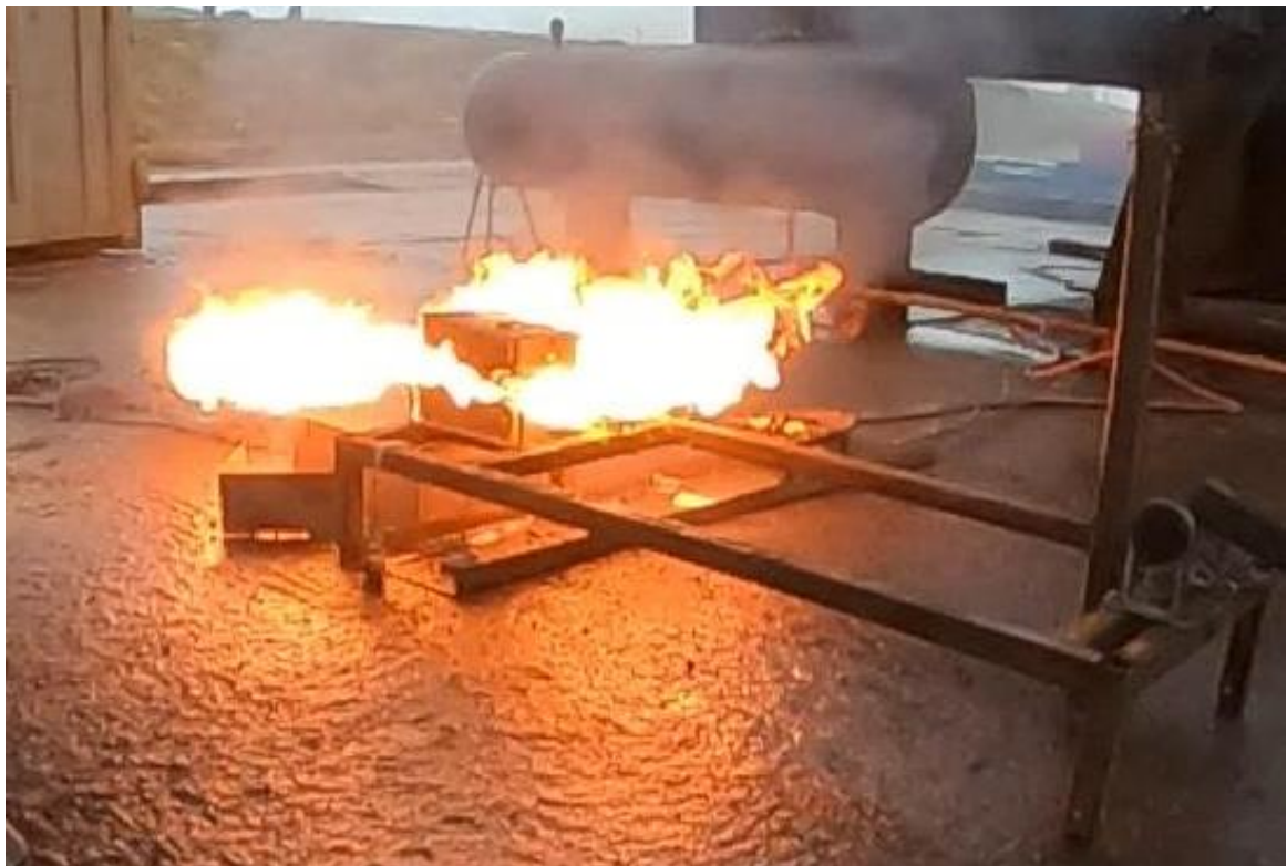
(j) A photograph of the rear of the modules when flare-like flames were observed (time = 46.2 s).
