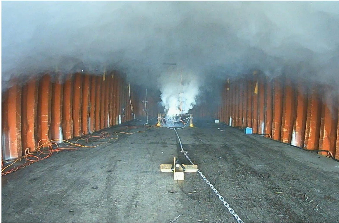
(e) A photograph taken during experiment C4 when a second type of vapour is emitted from the module, this sinks to the floor of the container suggesting it is heavier than air (time = 64.9 s).
