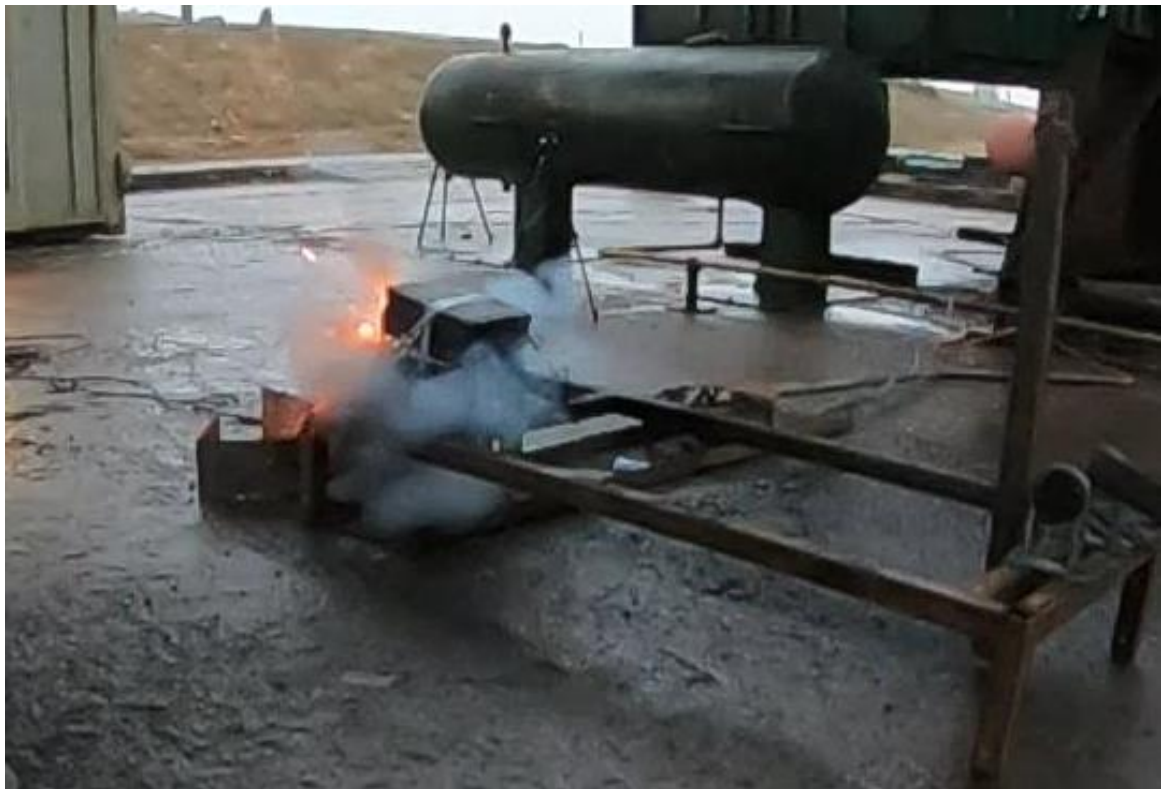
(f) A photograph of the rear of the modules when projectiles were first noticed to be emitted (time = 87.5 ms).
