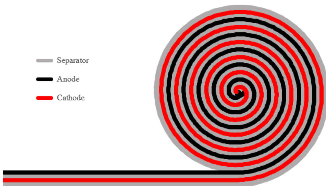
Figure 1.2. A schematic showing the components rolled in a cylindrical can.
