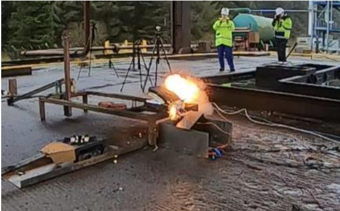
(i) A photograph of the front of the modules during ignition (time = 125 ms).
