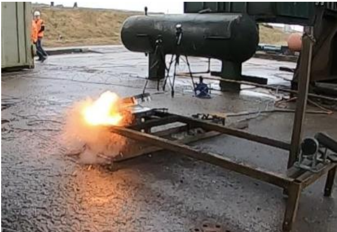
(j) A photograph of the rear of the module during ignition (time = 125 ms).
