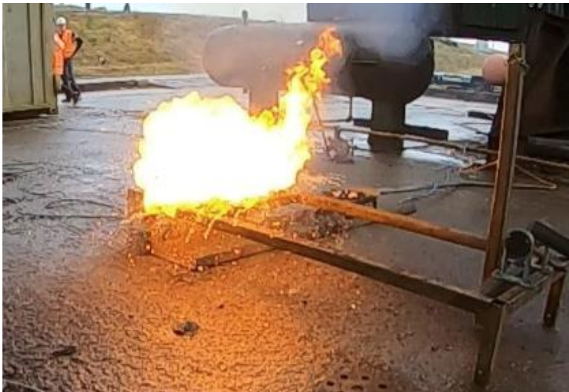
(l) A photograph of the rear of the module once flare-like flames had developed (time = 10 s).
