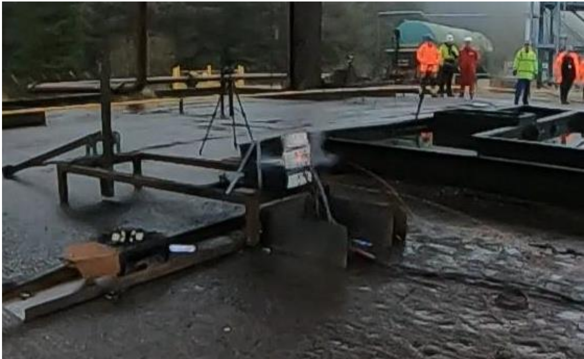
(c) A photograph of the front of the modules when ignition first occurred (time = 8.3 ms).
