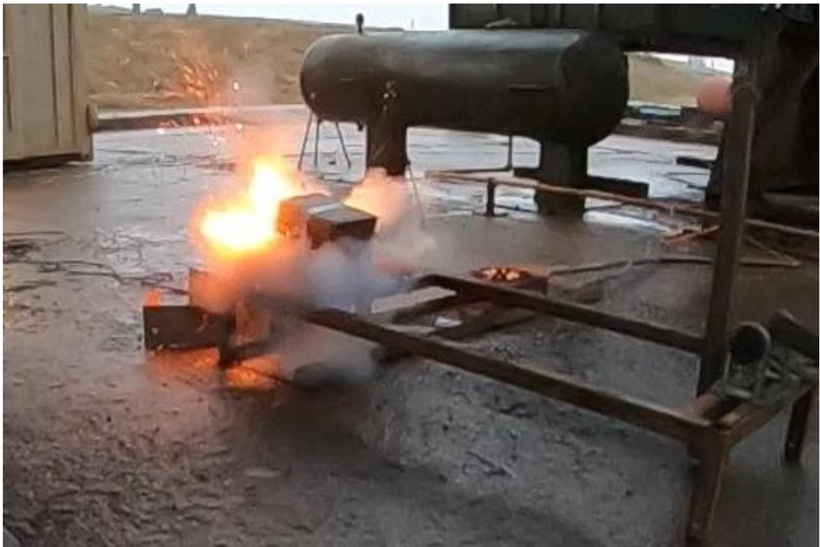
(h) A photograph of the rear of the modules when flames were first noticed (time = 154 ms).
