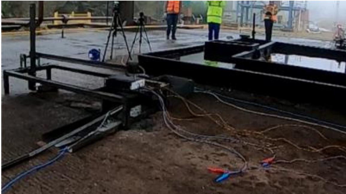
(a) The nail has just touched the module case commencing the experiment (time = 0 s).
