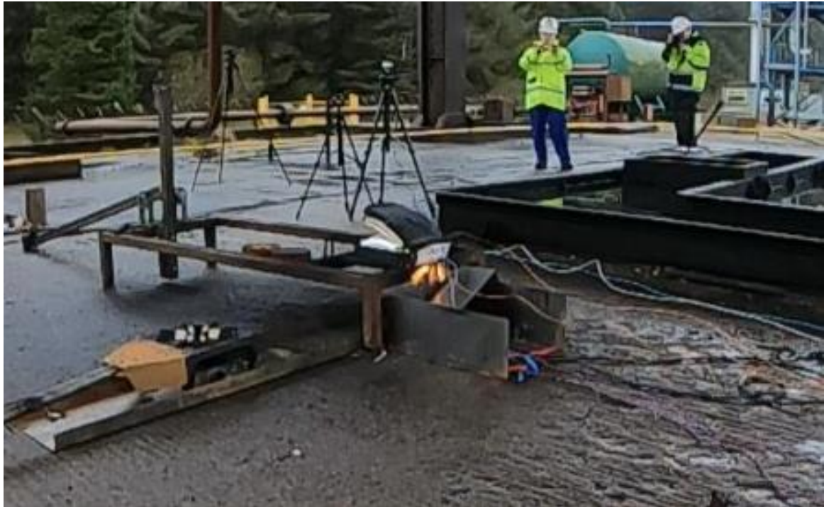
(c) A photograph of the front of the module when the module had been forced open (time = 45.8 ms).
