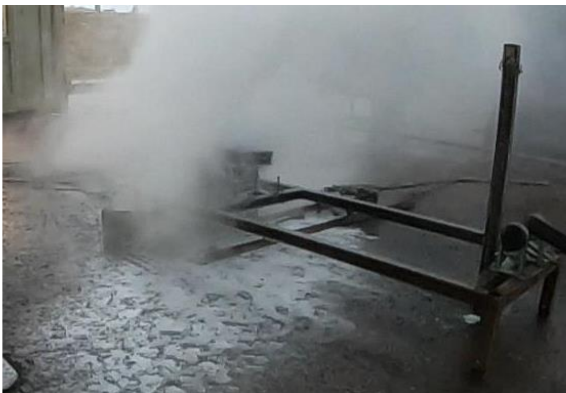
(l) A photograph of the rear of the modules once the flames had been extinguished and a dense white vapour cloud had been produced (time = 119 s).
