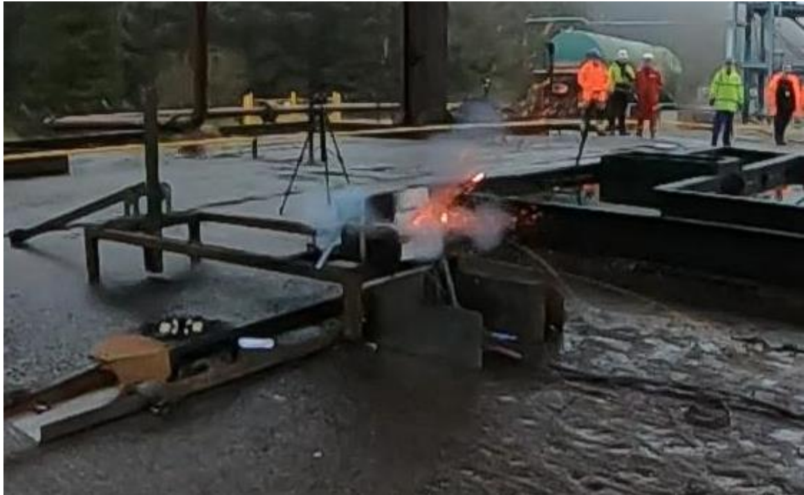
(e) A photograph of the front of the modules when projectiles were first noticed to be emitted (time = 87.5 ms).
