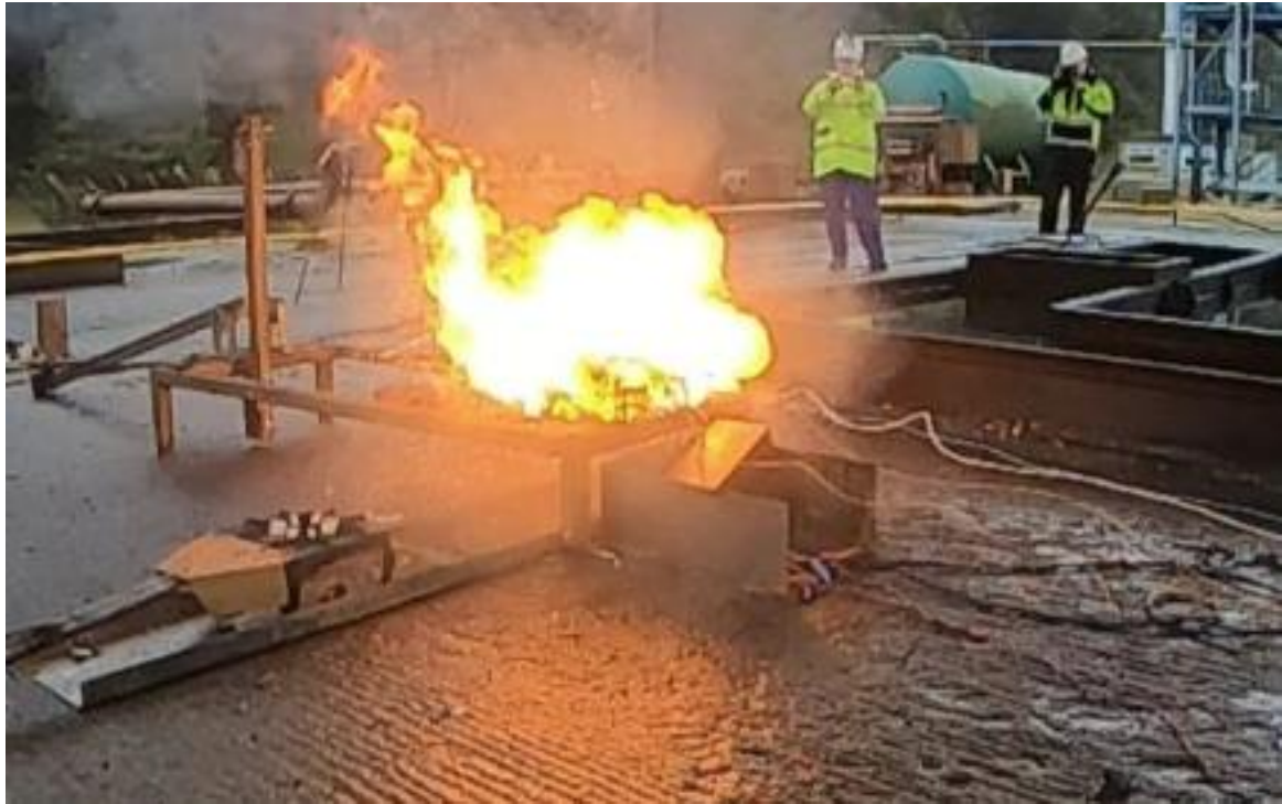
(k) A photograph of the front of the module once flare-like flames had developed (time = 10 s).
