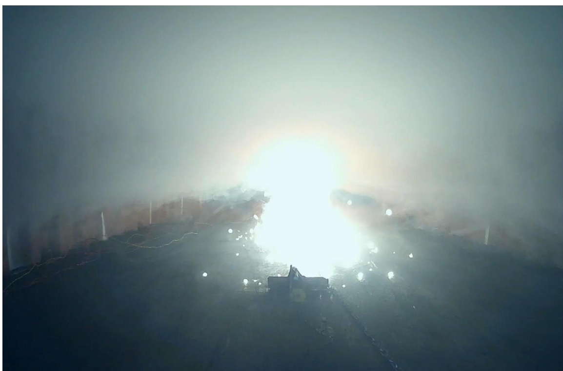
(h) A photograph taken during experiment C4 when the squibs are activated in an attempt to ignite the remaining vapour cloud (time = 120 s).
