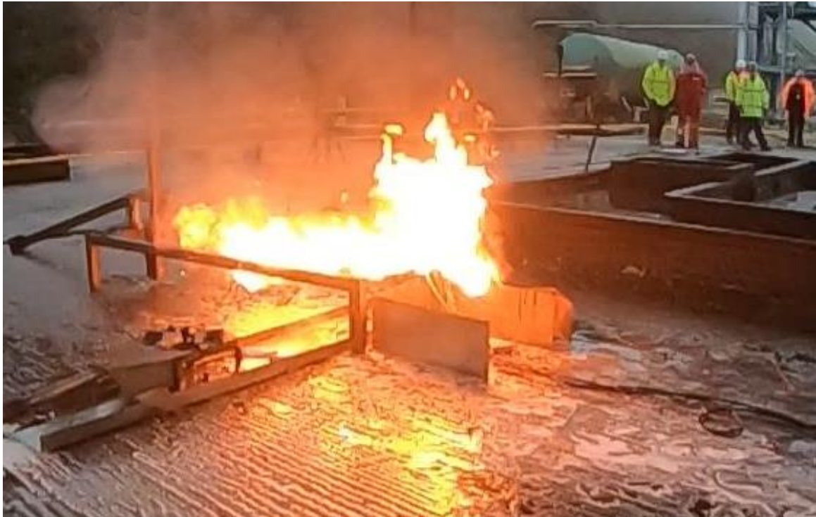
(o) A photograph of the front of the modules as flare-like flames were re-produced after extinguishments (time = 257 s).
