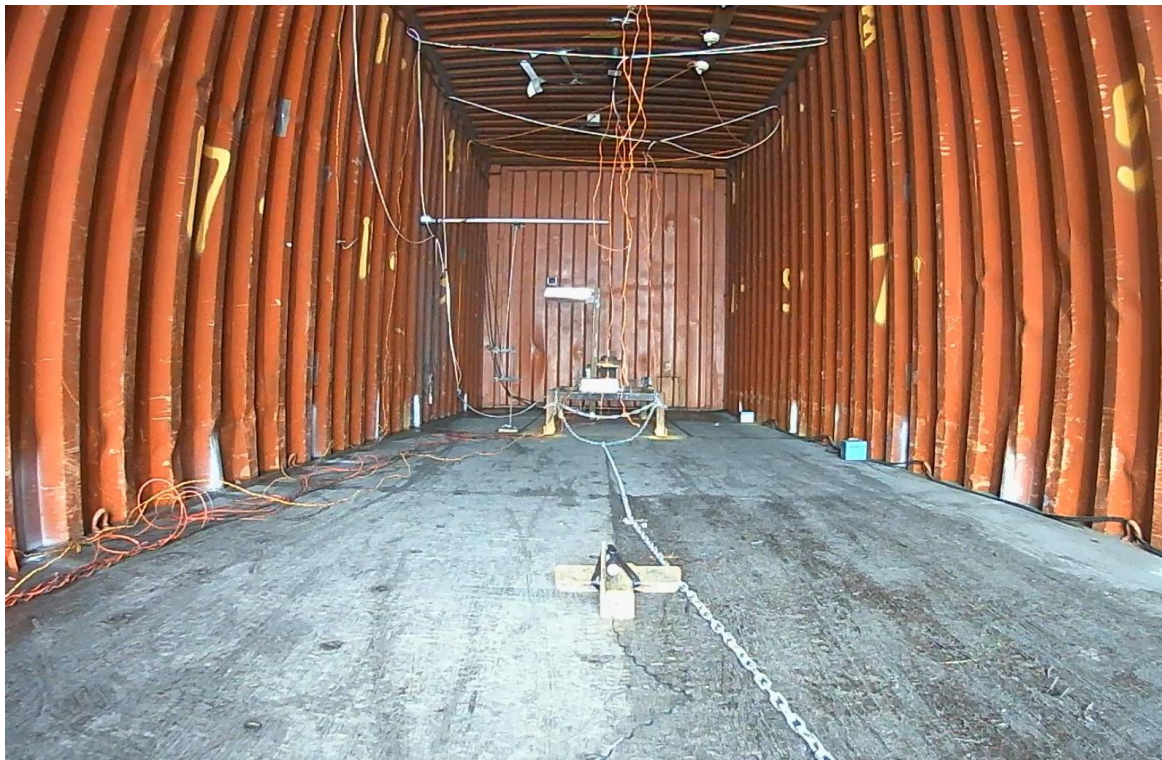
(b) A photograph taken during experiment C4 when a white vapour cloud began to be vented from the right hand side of the module (time = 1.33 s).
