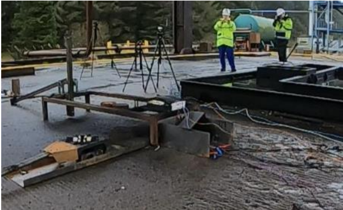
(a) A photograph of the front of the module when the pouch cells gassed, and the aluminium module case expanded (time = 0 s).
