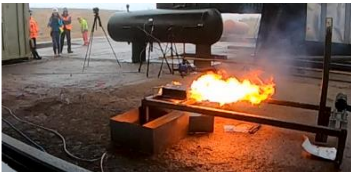
(b) Flare-like flames are observed 130 ss after the introduction of the burner.
