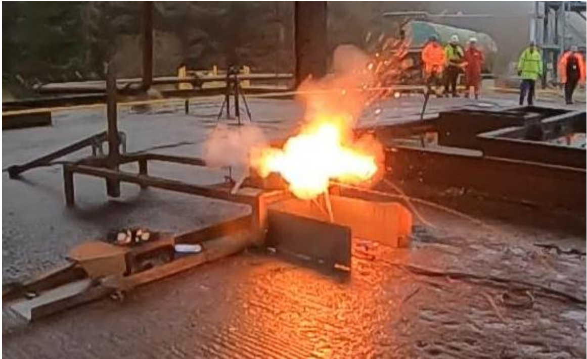
(g) A photograph of the front of the modules when flames were first noticed (time = 154 ms).
