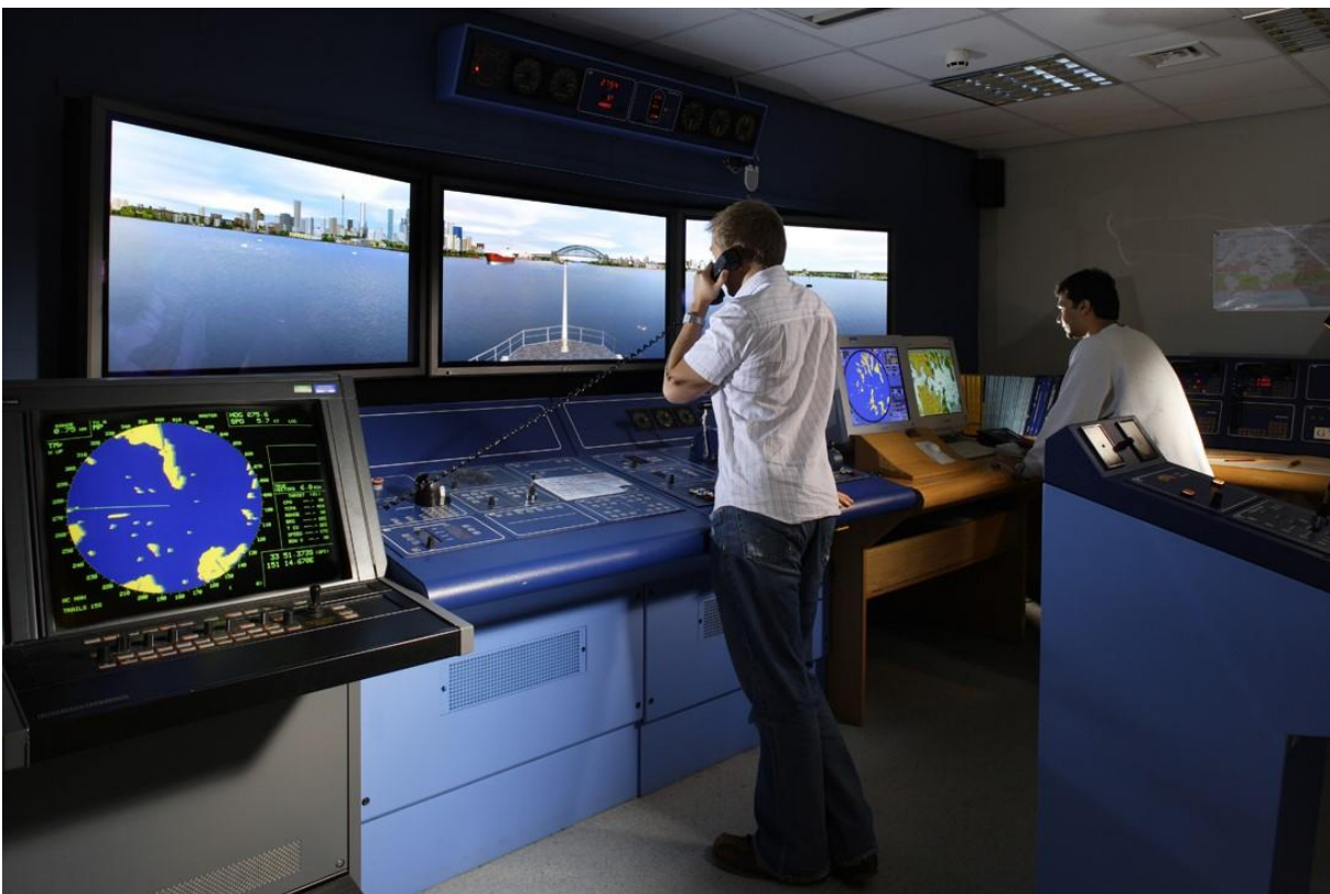
Figure 6.6.1 Bridge watchkeeping simulator configuration
