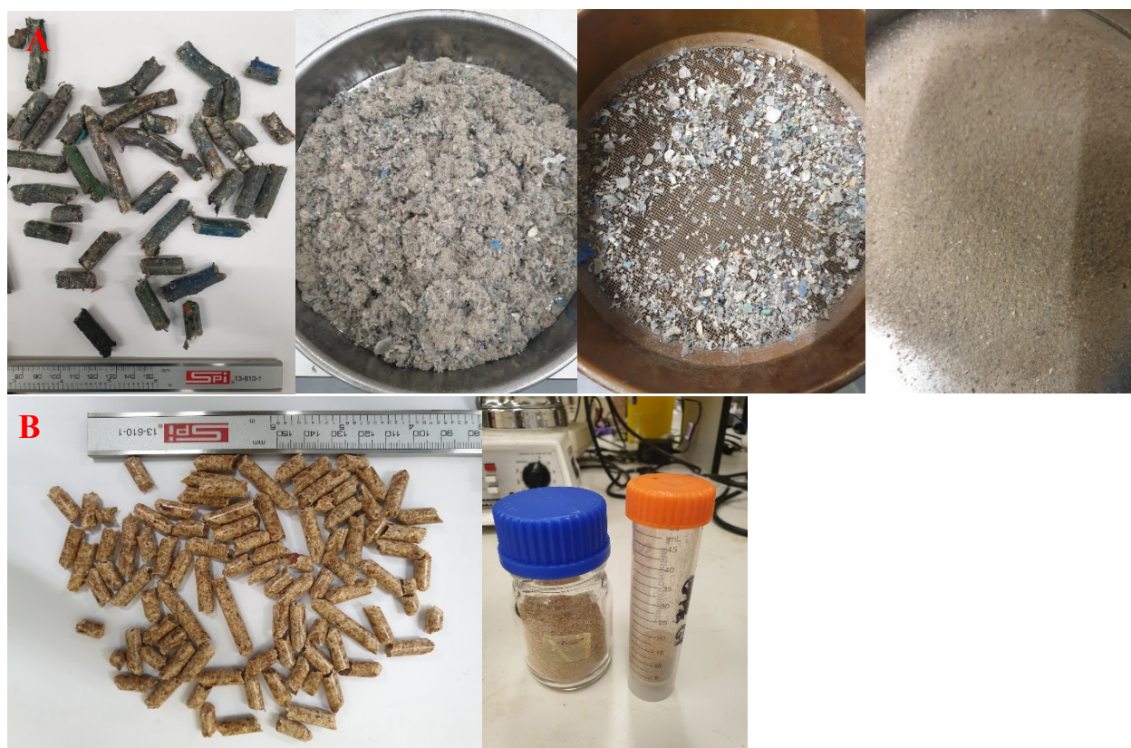
Figure 3.2: A.) Refuse-Derived Fuel (RDF) and B.) Waste wood pellets (WP), which has been reduced to a size of 2 mm for subsequent analysis.
