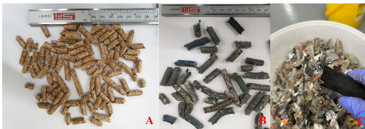
Figure 3.1: Waste used in this study including A.) wood pellets, B.) RDF pellets, and C.) RDF shreds.
