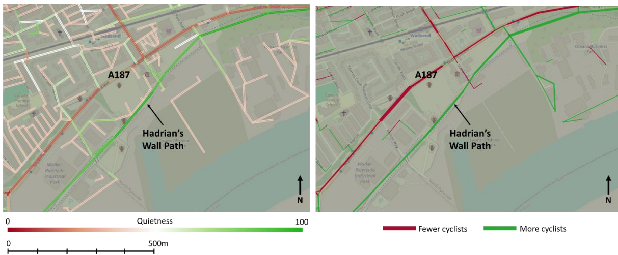
Figure 80 Comparison between the cycleability rating or quietness (left) and the differences between the number of cycling agents when the updated bicycle extension is enabled and disabled (example 3).
