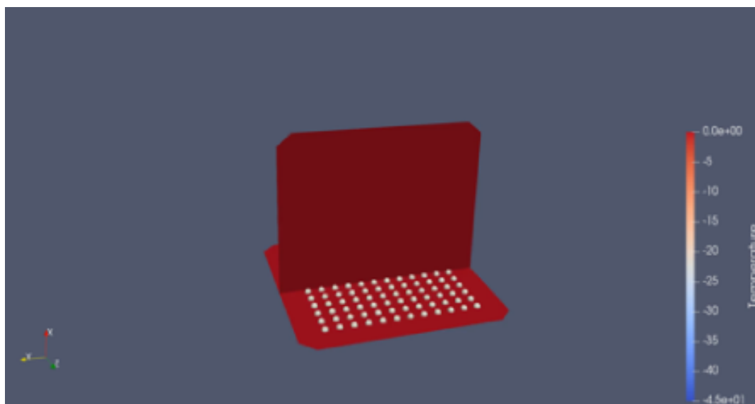
Figure 4.10: Simulated freezer space in CryoDynaMo with a freezing plate across the bottom of the simulation space.
