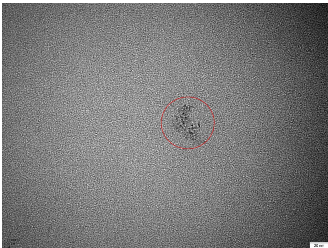
Figure 4.27 - TEM image of carbon dots (Ratio-20-CD) synthesised from precursor (Ratio-20-PT) (~20°C, 0.05/mL TA, 10/20 biomass ratio) - Scale Bar 20nm
