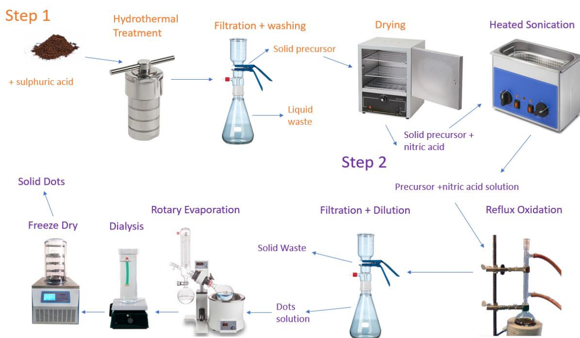
Figure 3.2 - The reaction schematic of two step carbon dot synthesis; hydrothermal carbonisation of coffee grounds followed by a nitric acid oxidation
