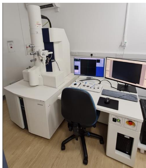
Figure 3.10 - Newcastle University's Hitachi HT7800 120kV Cryo TEM
