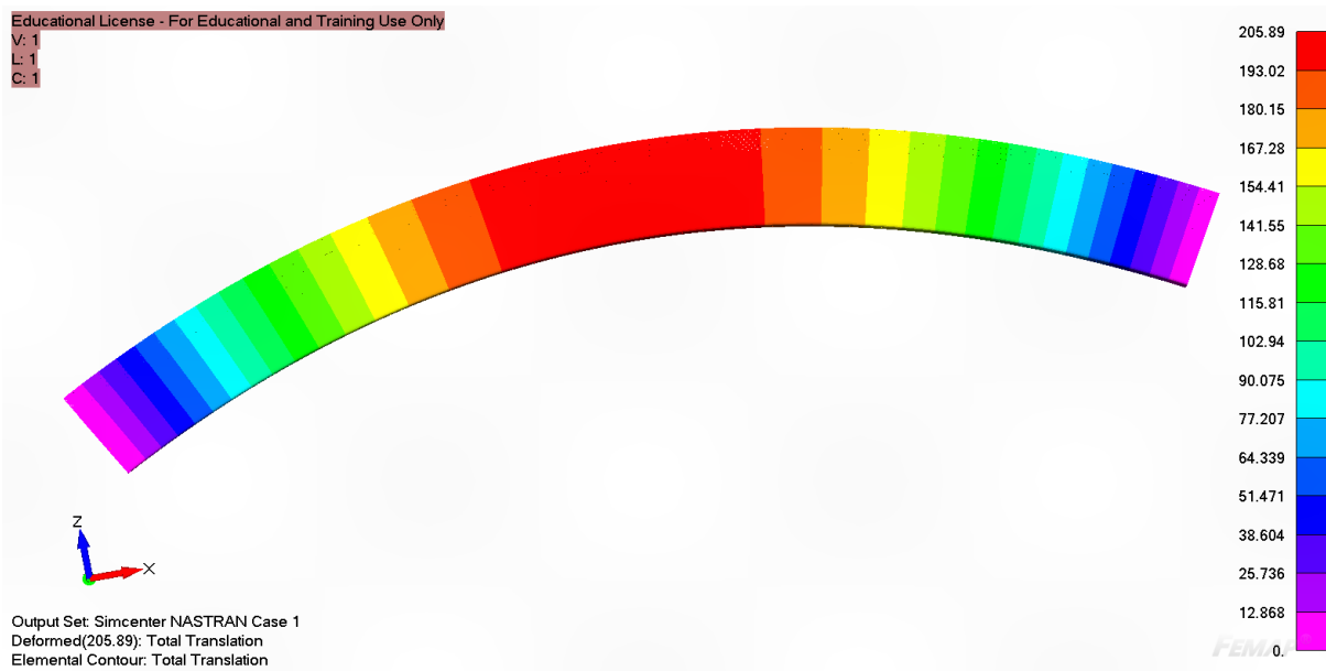
Figure 4-10: Longitudinal hull girder deflection (mm) along the ship's length (Hogging Head Sea).
