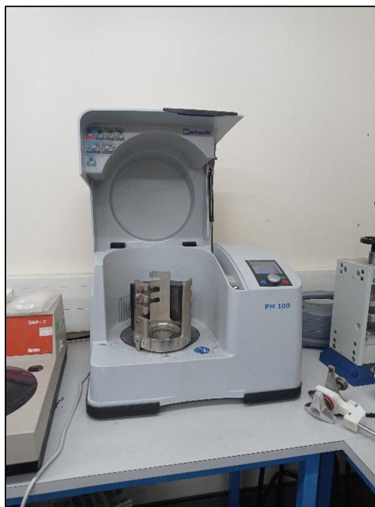
Fig. 4. 5 Overview of the tools and machine adopted for the sample preparation process: a) set of 6 agate grinding balls of varying sizes and grinding jar; b) a Planetary ball mill (PM100); c) approximately 7g of powdered sample ready to be loaded (sample ORTB 21).
