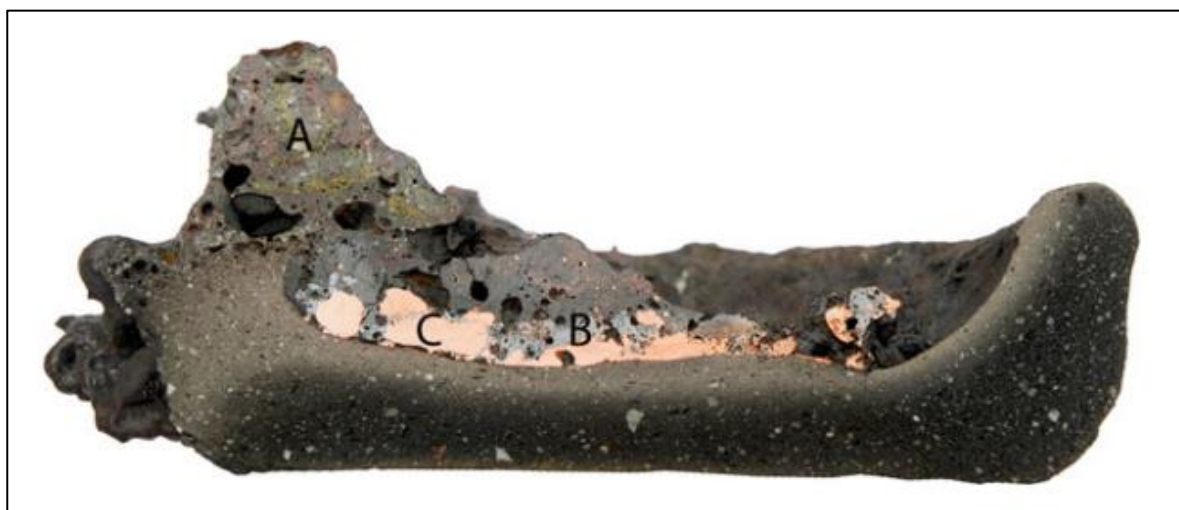
Fig. 7. 2 In the sectioned crucible three distinct layers were identified: (A) slag mixed with the melted ceramic body and finely interspersed copper prill; (B) a grey-silvery shining layer of matte with lamellae of bornite and chalcocite; (C) globules and accumulation of metallic copper, partly mixed with slag (From Hanning et al., 2010, p. 296, Pl. III. Experiment 14 (ore: Mercês I, P04c). Crucible width: 11 cm).
