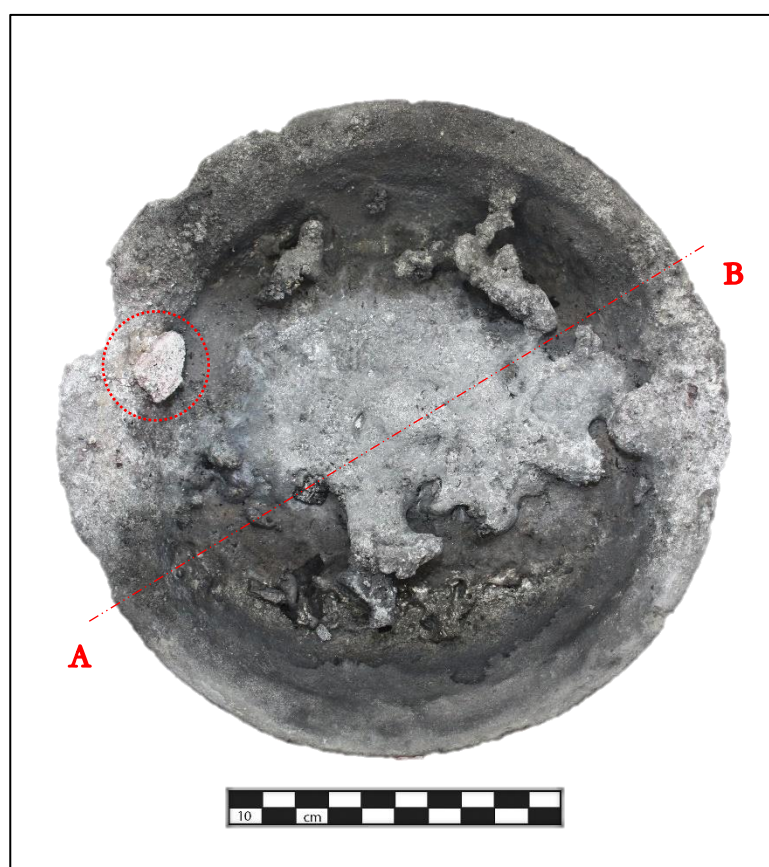
Fig. 6. 8 a) Top view of the crucible from Pilot experiment JH2021_PE_Exp.3_F.2. Three different layers were identified: 1) an upper layer characterised by a greyish, porous, and slag-like appearance; 2) just beneath the top layer, there is a combination of greyish and reddish shining layers, giving off a shining quality; 3) the lowest layer exhibits a noticeable gleam and is rich in copper content. Within the crucible, marked by a red dotted circle, one can also identify an unreacted piece of bornite. b) the cross-sectional view A-B of the crucible reveals the products obtained during the experiment, which are scattered across the crucible's surface.
