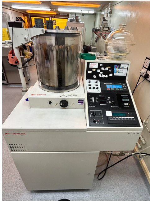
Figure 2.9: The Edwards 306 e-beam evaporator used for this research.
