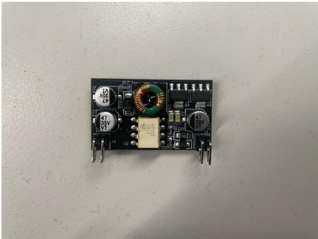
Fig 5.5 PCB prototype of the second gate driver
