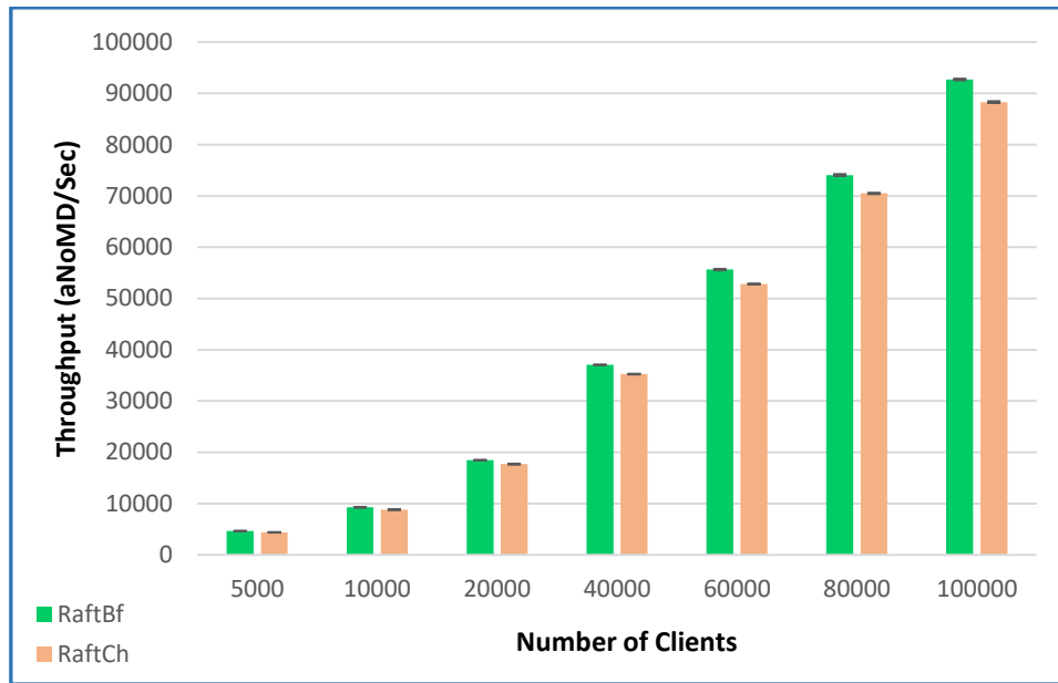
Figure 6.10 Throughput Comparison for RaftBf and RaftCh (Non-Zero Processing Delay)
