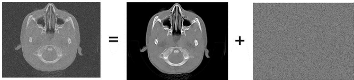
Figure 2.3. A noisy image is the sum of the clean image and the noise component (adapted with permission from Diwakar and Kumar (2018)).
