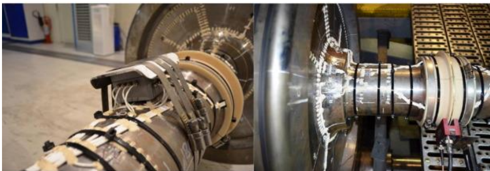
Figure 2.7 The wheelset instrumented with telemetry system (top) under preparation (left) and then on BU300 test rig (right) [15]
