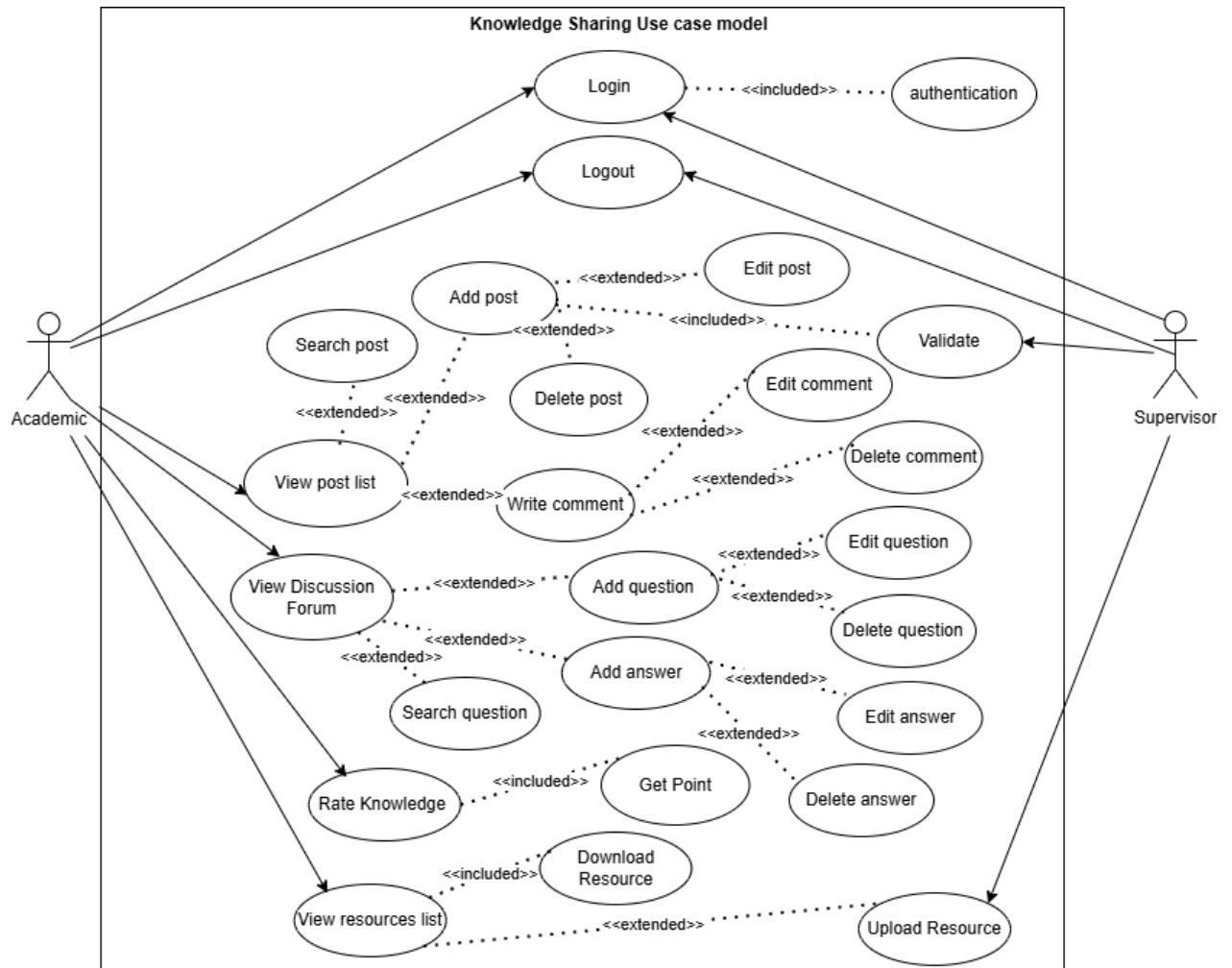
Figure 5.3 Use Case diagram of the TEP System
