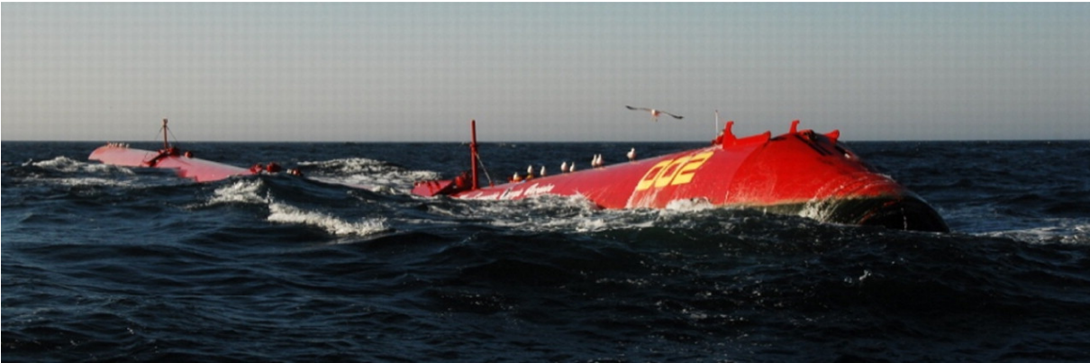
Figure 2.3: “Pelamis” WEC on site in Portugal [9].
