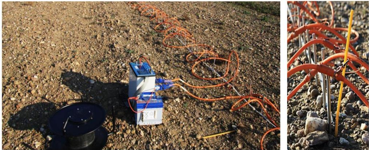
Figure 2. 2 ERT setup demonstrates an electrode array consisting of an electrical meter with cables and electrodes (Wiekenkamp, 2012).
