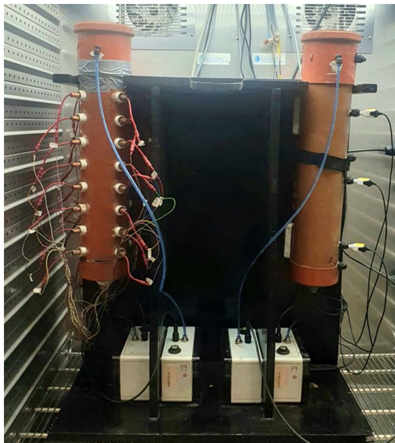
Figure 3. 4 A photograph of the soil column experiment contained in the environment chamber at the NGIF.
