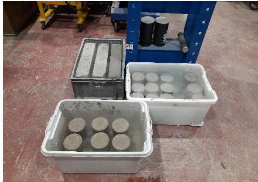
(o) Curing process of the samples
