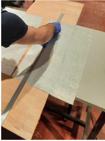
(c) Preparation of GFRP fabrics
