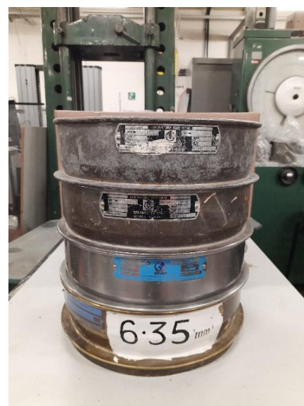
(b) Sieve sizes for coarse aggregates
