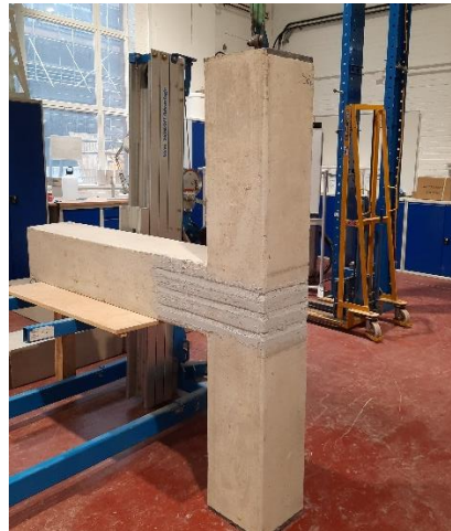
(j) Filling the groove with epoxy adhesive and levelling the surface.
