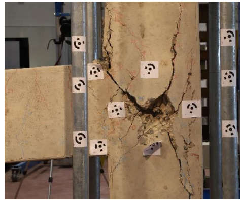
(i) Drift ratio: 5.77%, Displacement: 75 mm
