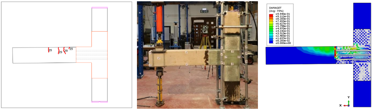
(a) Drift ratio: 0.92%, Displacement: 12 mm
