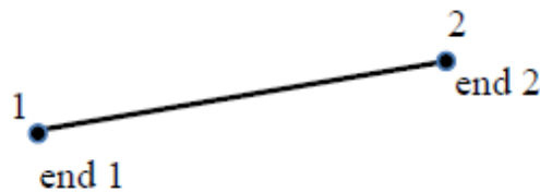
Figure 5.3. T3D2 (2-node, 3-dimensional truss element) (Abaqus Analysis User's Guide, 2016).
