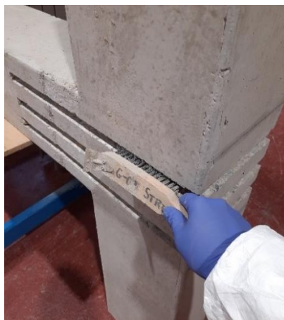
(e) Cleaning the grooves with a wire brush.
