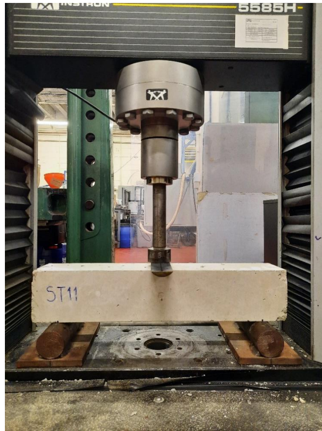
Figure 3.6. Three-point bending test of concrete.
