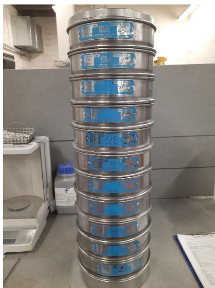
(a) Sieve sizes for fine aggregates
