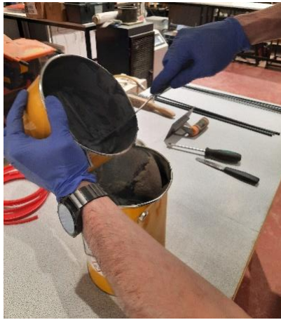
(g) Component A, which is white in colour, is mixed with component B, which is black.
