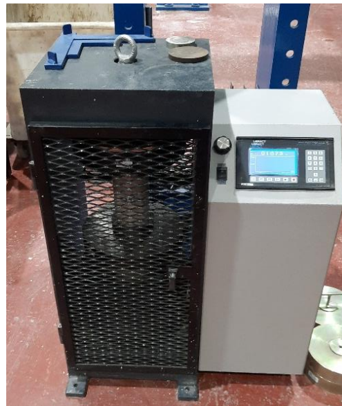
Figure 3.7. The test equipment for concrete compression strength.
