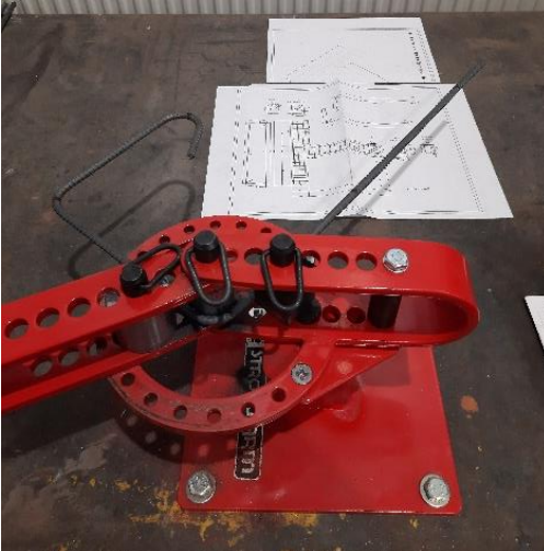
(c) Bending of transverse rebars
