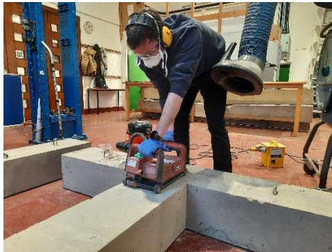
(c) Cutting grooves using reference drawings with Hilti DC-SE20.
