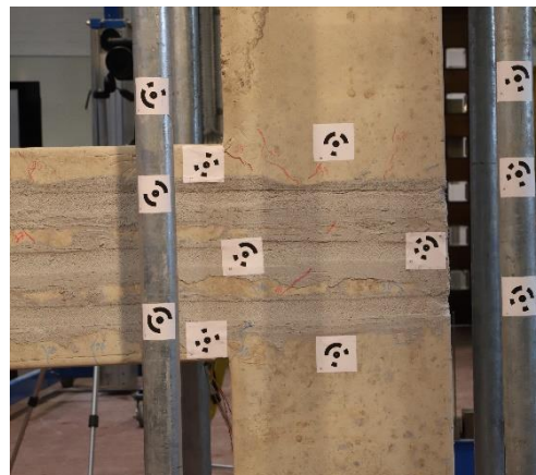
(e) Drift ratio: 2.31%, Displacement: 30 mm
