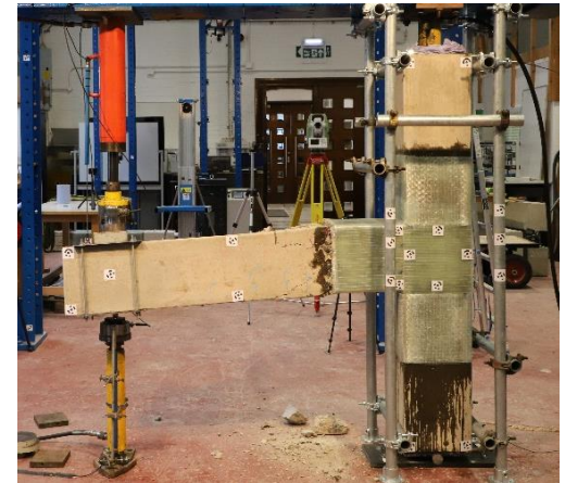
(f) Drift ratio: 5.77%, Displacement: 75 mm
