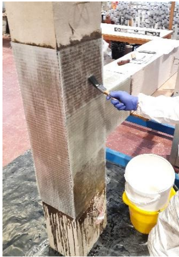
(e) Application of the adhesive material
