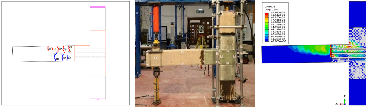
(b) Drift ratio: 1.54%, Displacement: 20 mm
