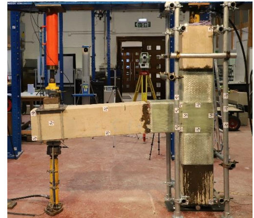
(e) Drift ratio: 4.62%, Displacement: 60 mm
