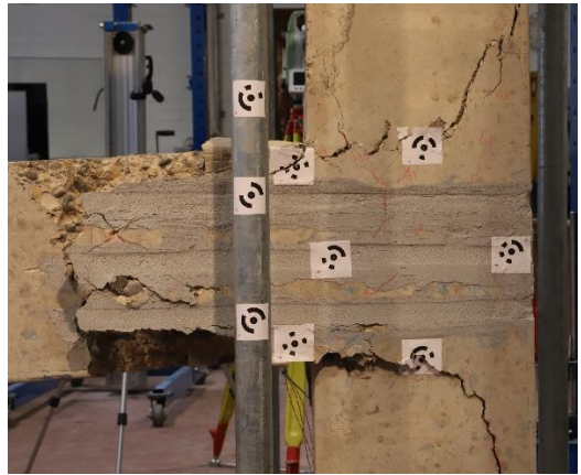
(h) Drift ratio: 5.77%, Displacement: 75 mm
