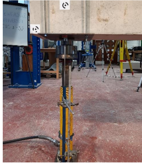
(b) LVDT location at the bottom of the beam
