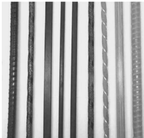
Figure 2.10. Types of FRP bars for NSM applications (De Lorenzis and Teng, 2007).
