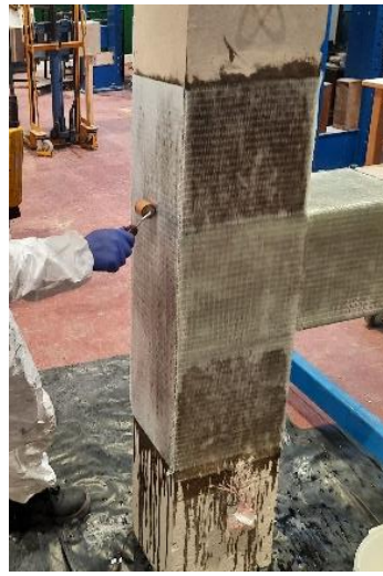
(f) Uniform distribution of the adhesive material
