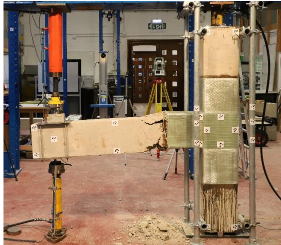
(h) Drift ratio: 7.31%, Displacement: 95 mm
