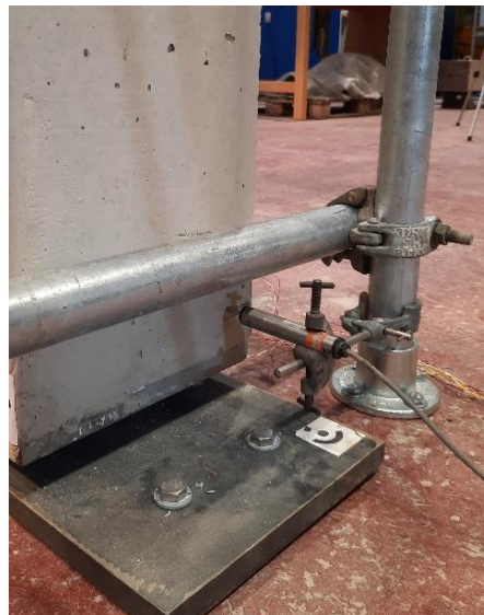
(b) LVDT location at the bottom surface of the column
