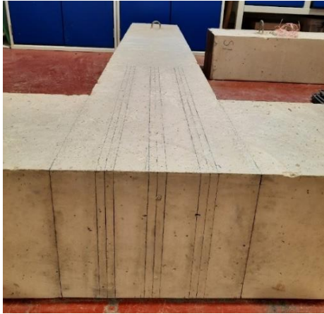
(a) The reference drawings before cutting the grooves for the NSM method.
