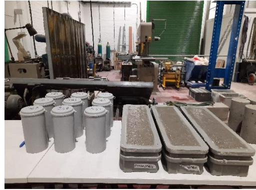
(n) Samples taken during the concrete pouring process
