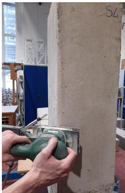
(a) Rounding of the corners to prevent stress concentration
