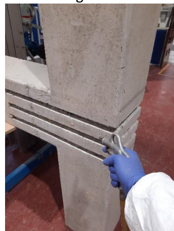
(f) Cleaning the grooves with a high-pressure air jet.
