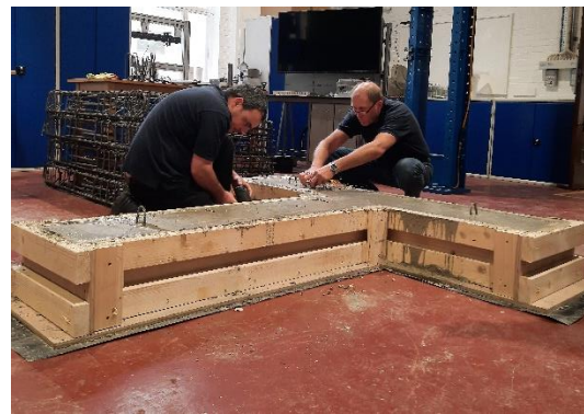
(l) Demoulding the specimen
