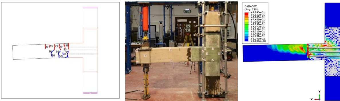
(c) Drift ratio: 2.31%, Displacement: 30 mm
