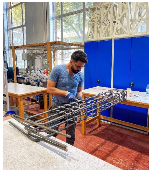
(f) Tying of the beam reinforcements
