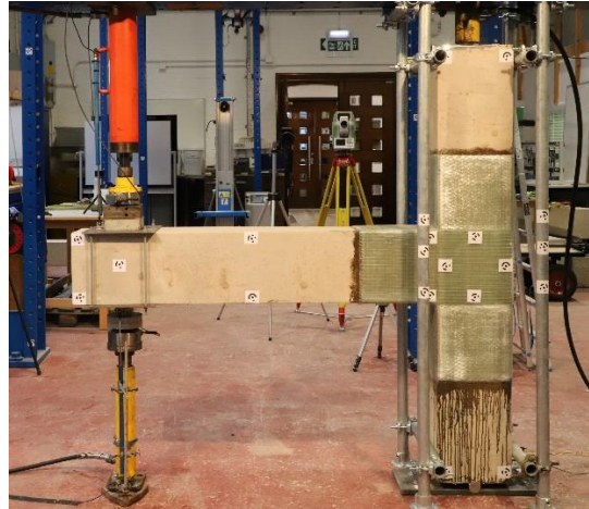
(a) Drift ratio: 0.92%, Displacement: 12 mm
