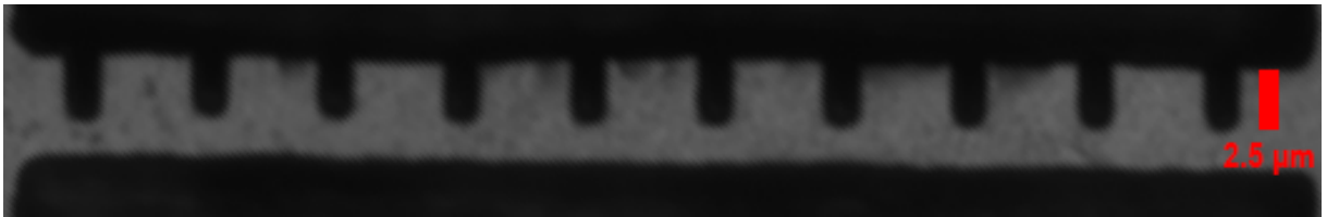
Figure 6.1 The emitter structures of emitter array C-H, as closely examined as possible via oil immersion, 488 nm confocal microscopy.
