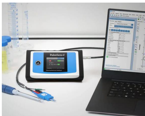
Figure 2.6: Photograph of potentiostat (electrochemical workstation), PalmSens4 (PalmSens, the Netherlands).
