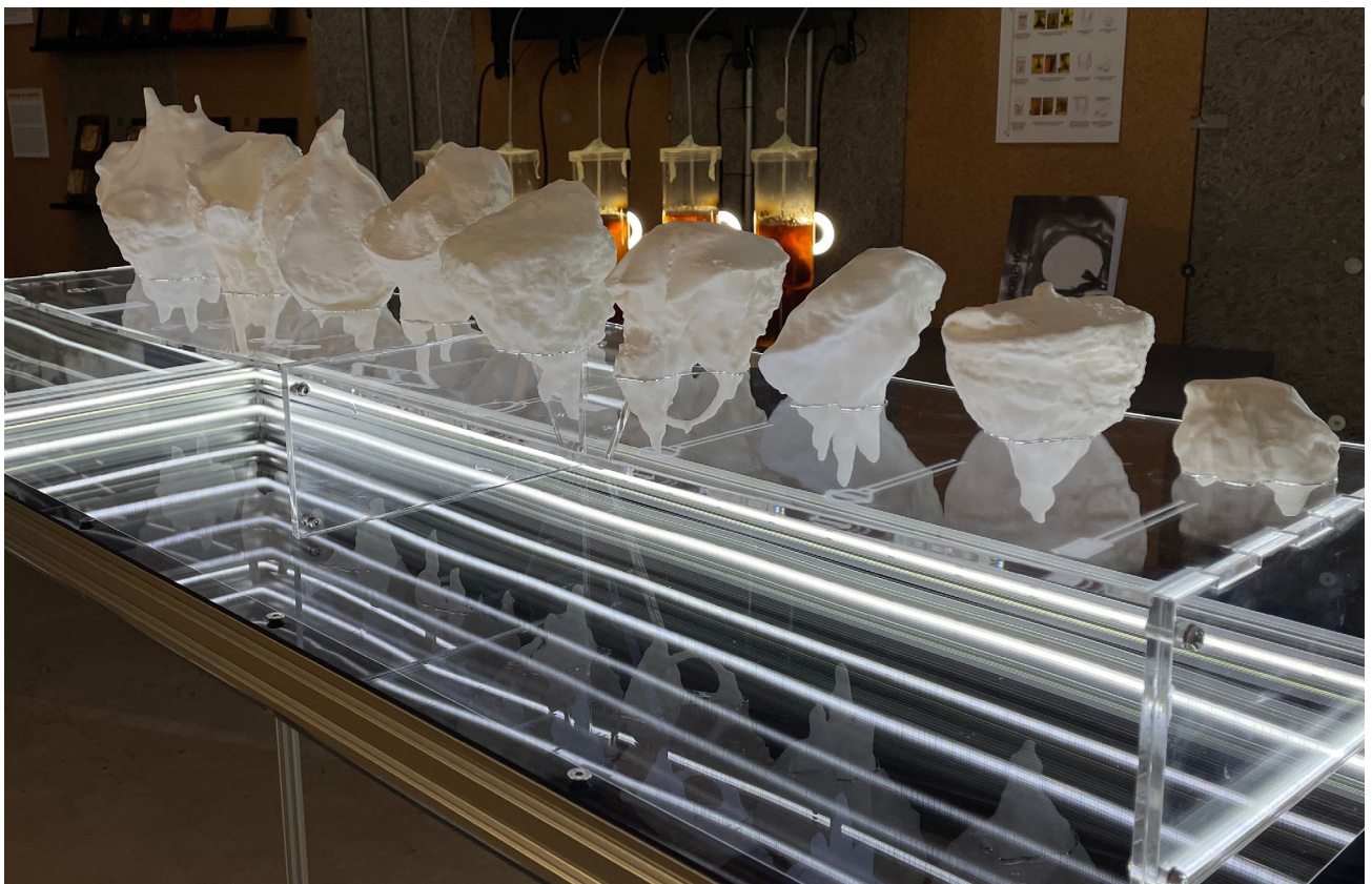
Figure A4: Representation of BC forms grown around various different aeration scaffolds. The forms are 3D printed based on 3D scan made of the frozen forms and the respective scaffold is etched into the clear stand.
