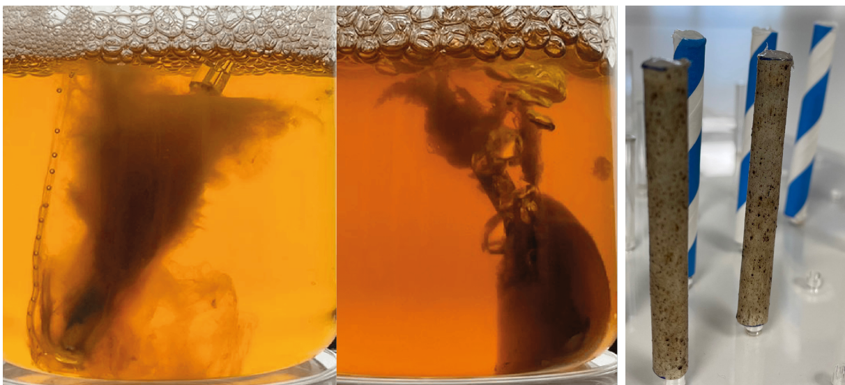
Figure 6.93: (left) Comparison of BC on paper straws extending the whole length of the straw and BC on bioplastic scaffold concentrated around the bottom end of the straw; (right) silicone glue sealing off the bottom end of the bioplastic straw
