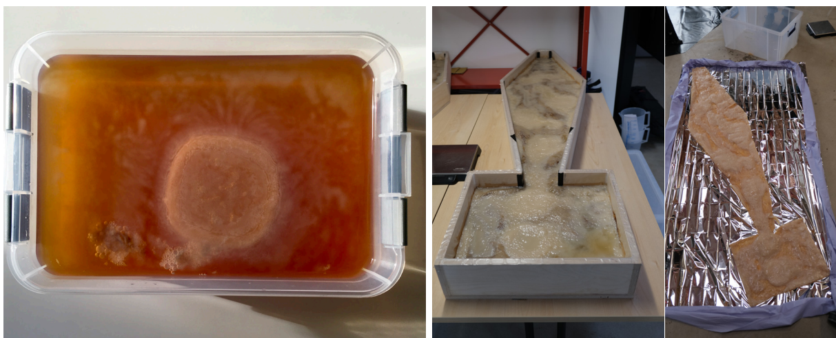
Figure 2.6: (left) Static culturing method of BC with SCOBY; (right) static culture with customised shape during growth and after harvesting
