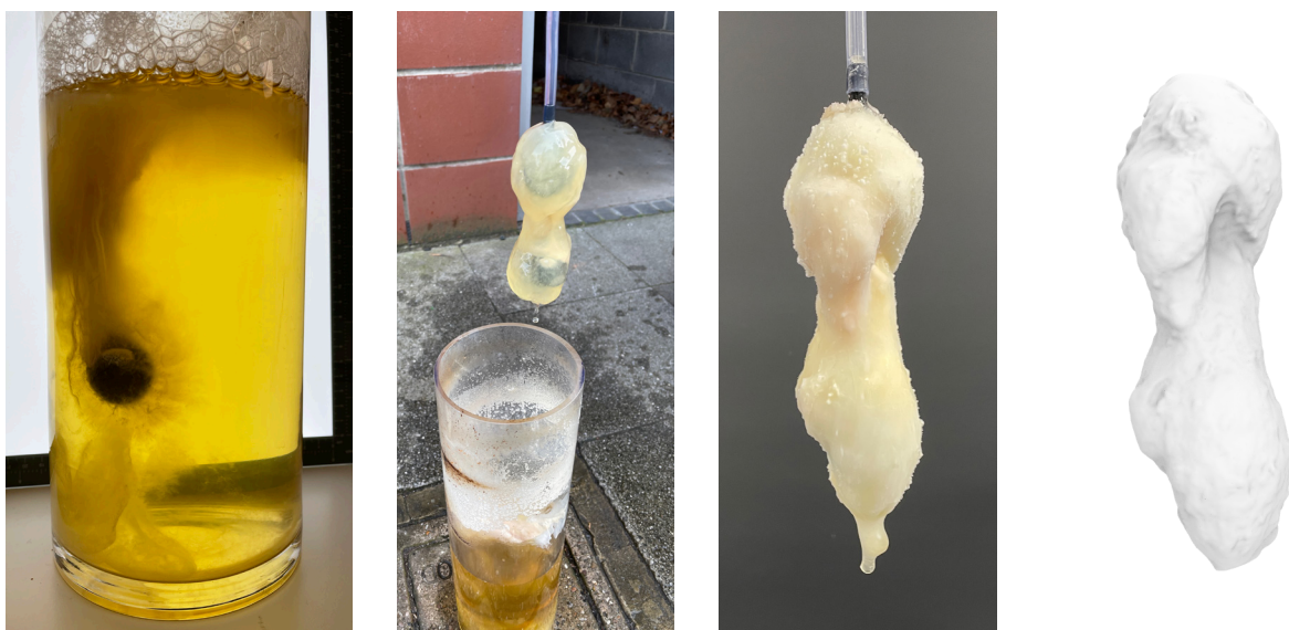
Figure 8.7: Example of immature BC detachig from the scaffold during harvest from Exp. P. (Left to right) Visible BC growth on day 11, harvest on day 18, the frozen BC form, and a digital render of the 3D scanned morphology
