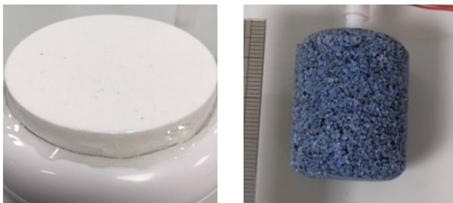
Figure 5.64: Visual difference in pore size of aeration disc (left) and air stone (right)
