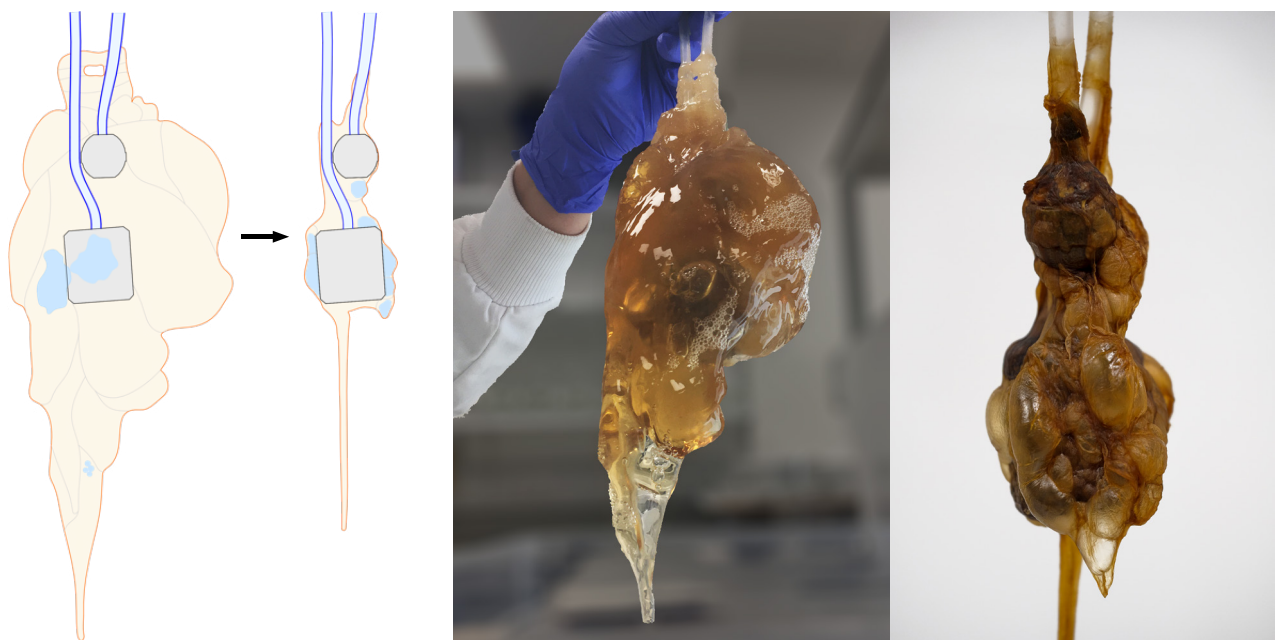
Figure 7.1: (Left) Diagram showing shrinkage of BC around scaffold with trapped air pockets in 5 days, (right) comparison of shape and volume of sample in hydrated and air-dried state after 7 days
