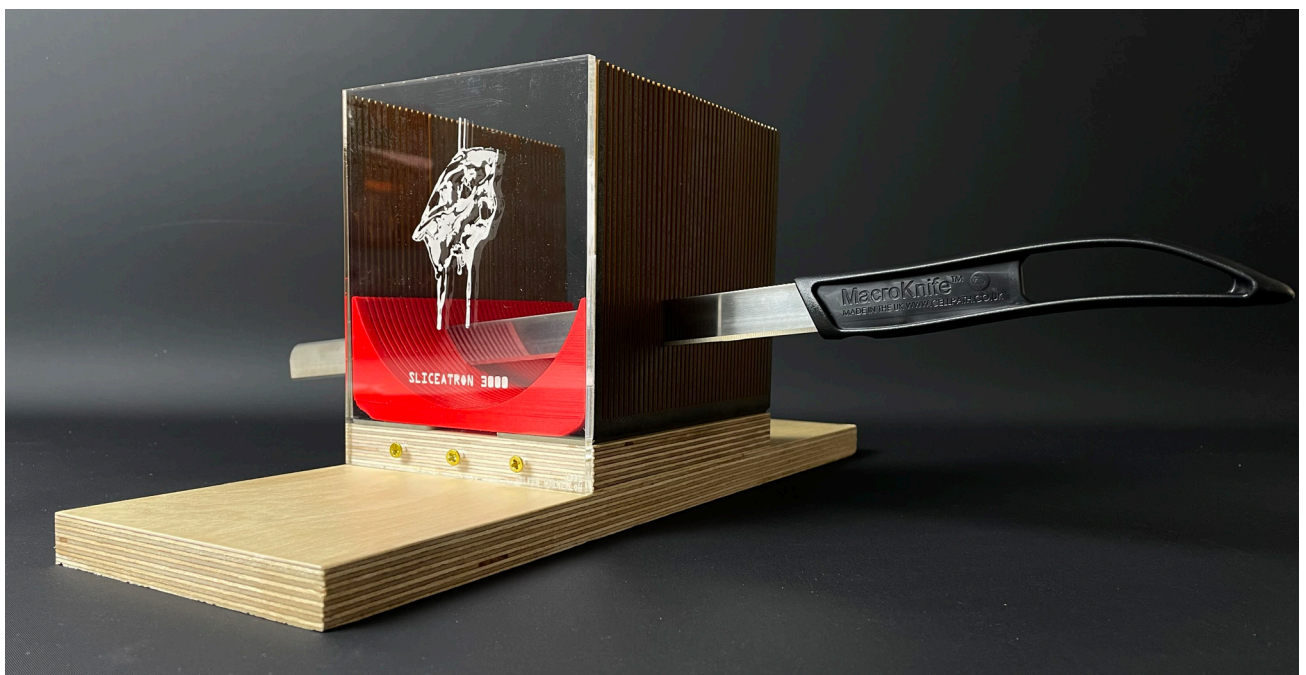
Figure 7.14: Custom-built slicing mould, Sliceatron 3000, to cut hydrated BC forms into slices
