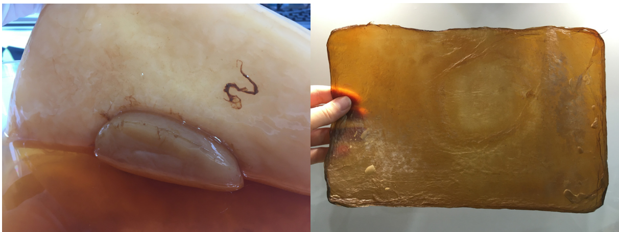
Figure 4.3: (Left) SCOBY attached to newly grown pellicle; (right) dried BC with visible material change where the SCOBY was attached
