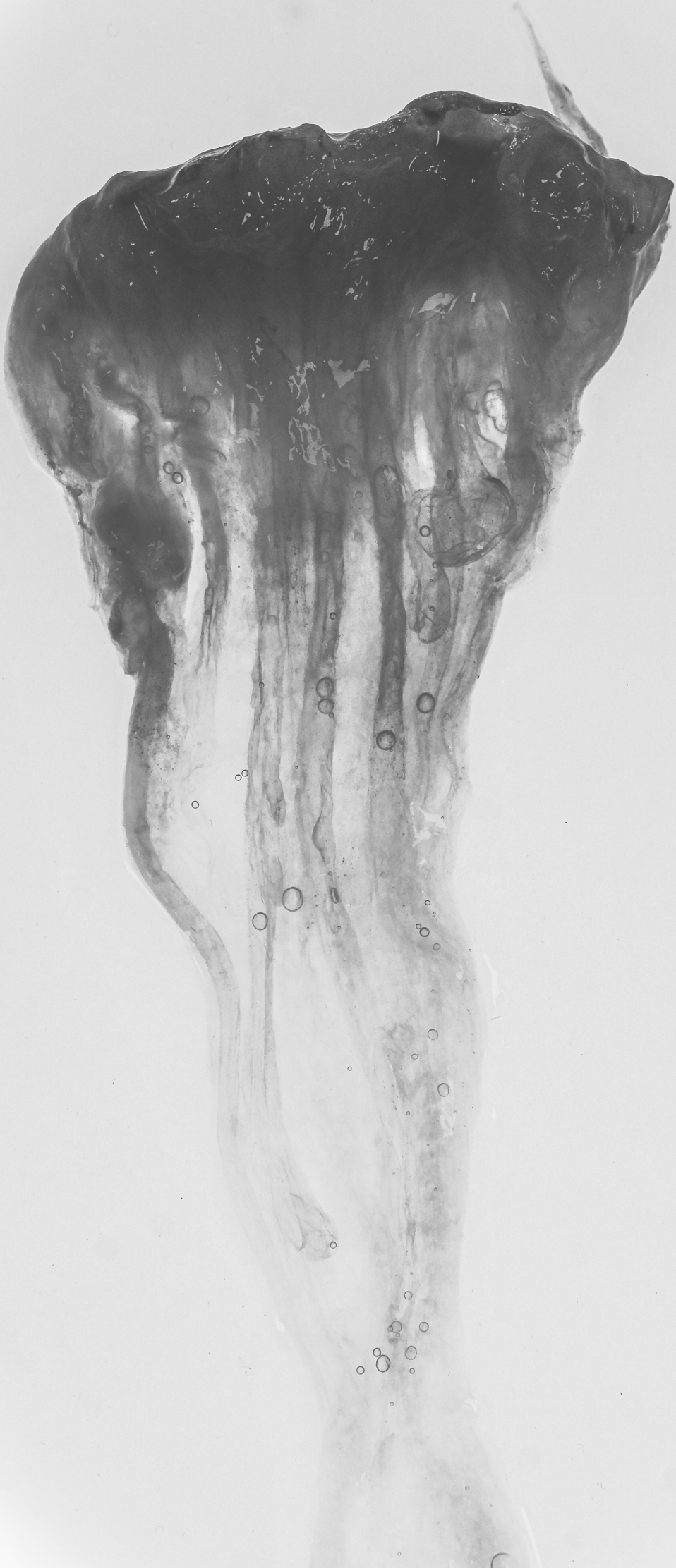
Bacterial cellulose grown with submerged aeration disc with distinct elongated growth features
