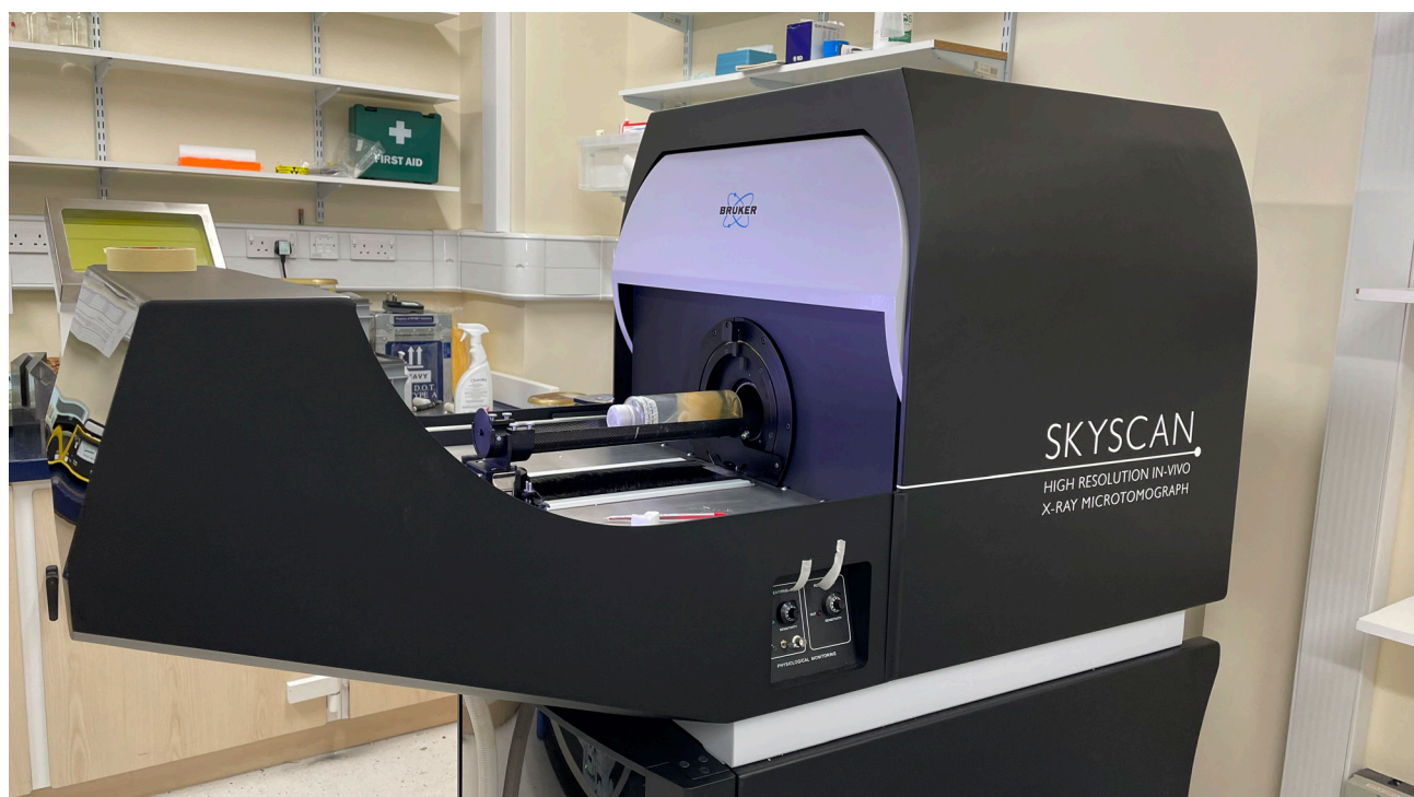
Figure 7.23: BC sample being tested inside the SKYSCAN CT machine for digital X-ray imaging
