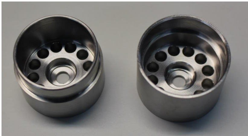
Figure 7-7: Two parts of machined motor outer housing
