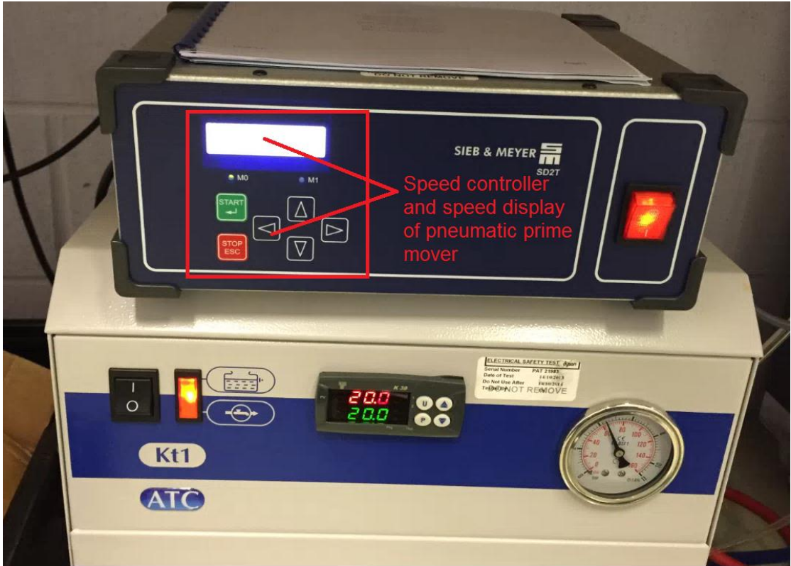
Figure 8-13: The utilised pneumatic prime mover with speed controller & display
