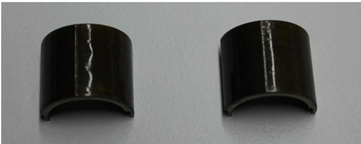
Figure 7-12: Two half-ring shape stator parts
