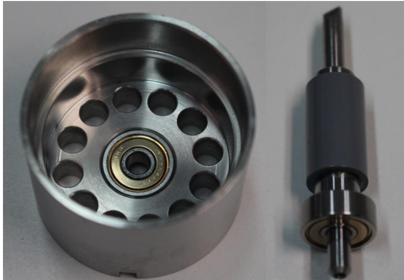
Figure 7-8: The assembled high-speed bearings
