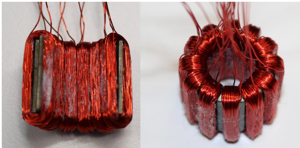
(a) Assembled half stator
