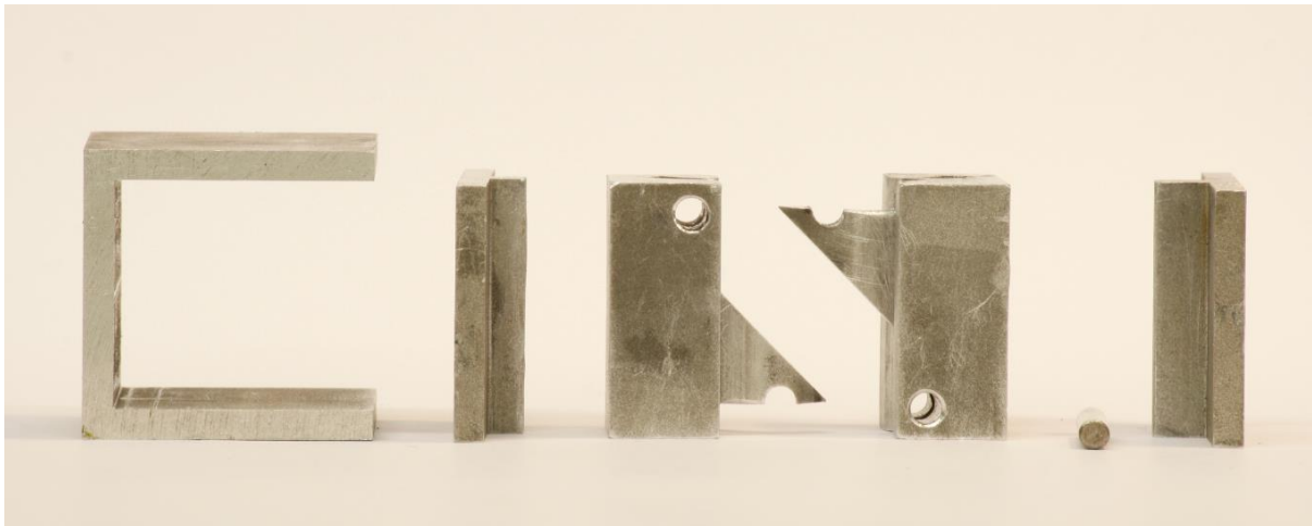
Figure 7-13: Components of the designed winding mould
