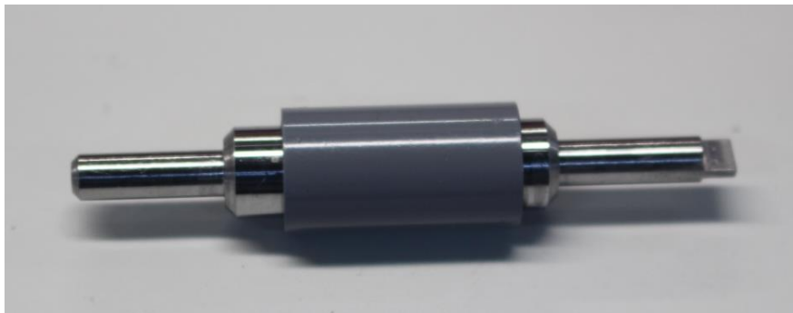
Figure 7-6: Fully assembled rotor
