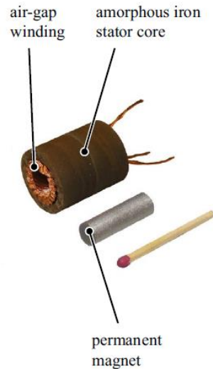
Figure 2-3: Comparison of manufactured motor components to a match [2]
