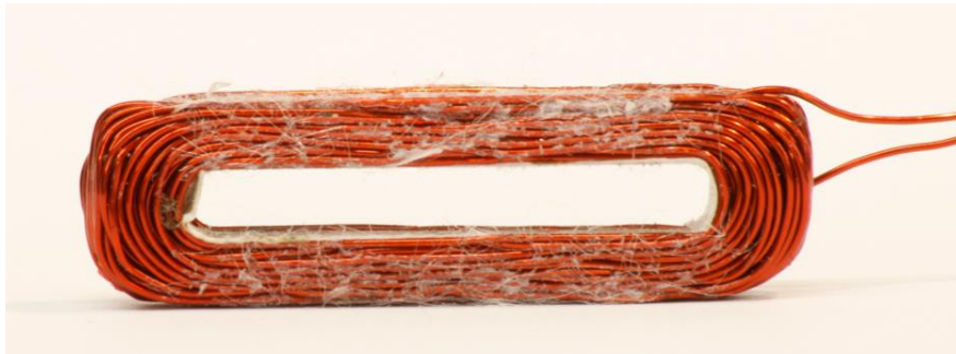
Figure 7-15: Actually built single toroidal winding coil
