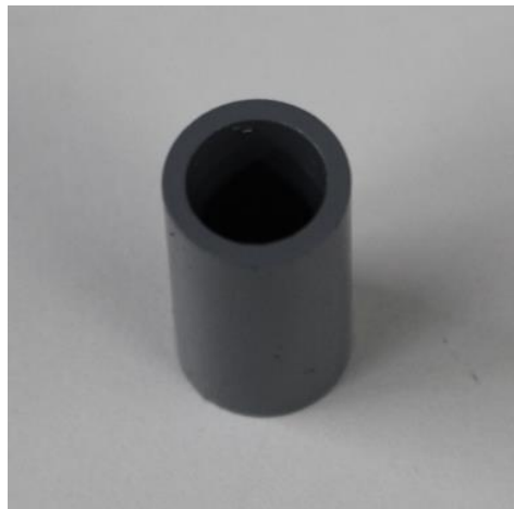
Figure 7-1: Produced ring-shape rare-earth permanent magnet
