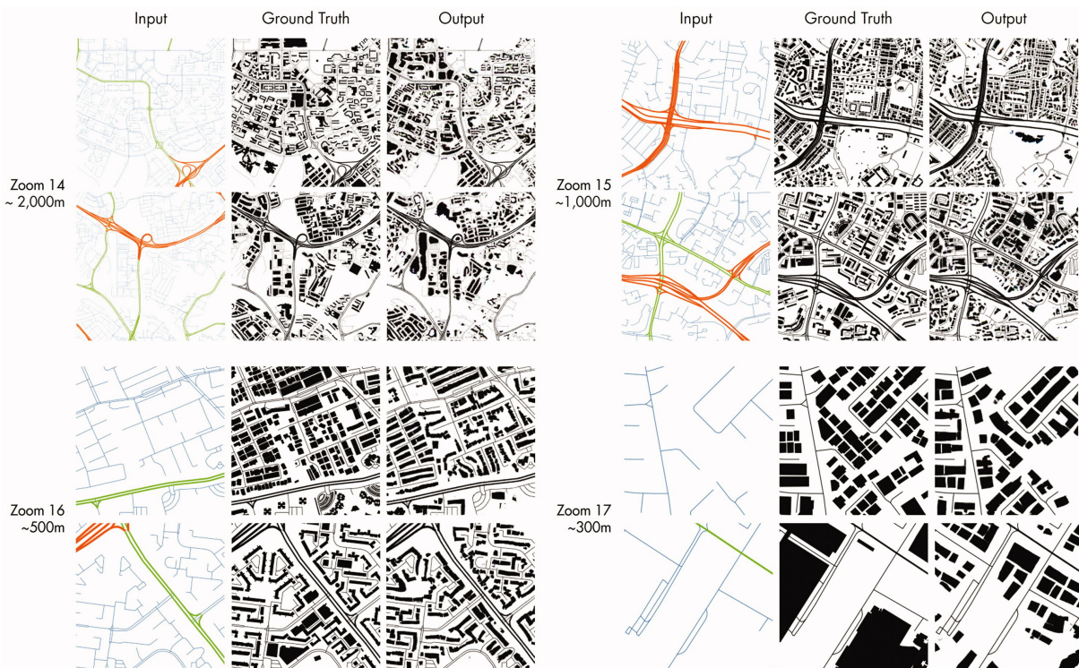
Figure 2.8: GANmapper building footprint outputs at four different zoom levels (Wu and Biljecki, 2022).
