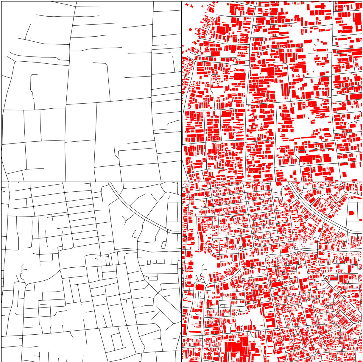
Figure 6.5: 500 m 2 (top row) and 1000 m 2 (bottom row) spatial scale of the building footprint images. Input image (left) and target image (right) at 1024x1024 resolution.
